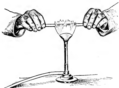
FIG. 5.—Bending a tube into a right angle—I.
