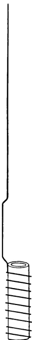
FIG. 27.—Combustion cup (or deflagrating spoon) made from a piece of copper wire and a piece of crayon having a cavity at the upper end.
