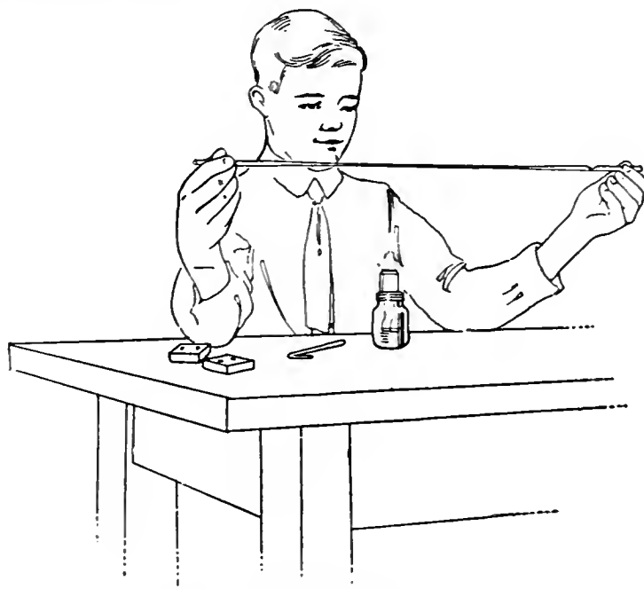
FIG. 16 DRAWING A THIN TUBE
