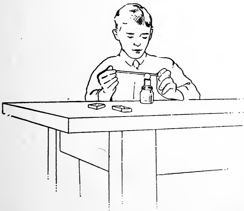
FIG. 3 HEATING GLASS TO SOFTEN IT
