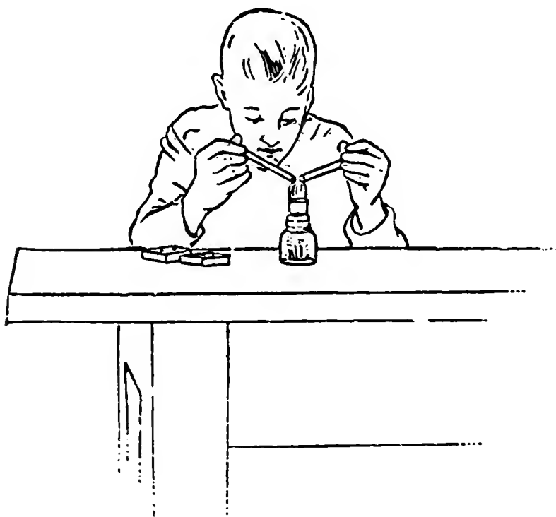
FIG. 72 JOINING TWO TUBES
