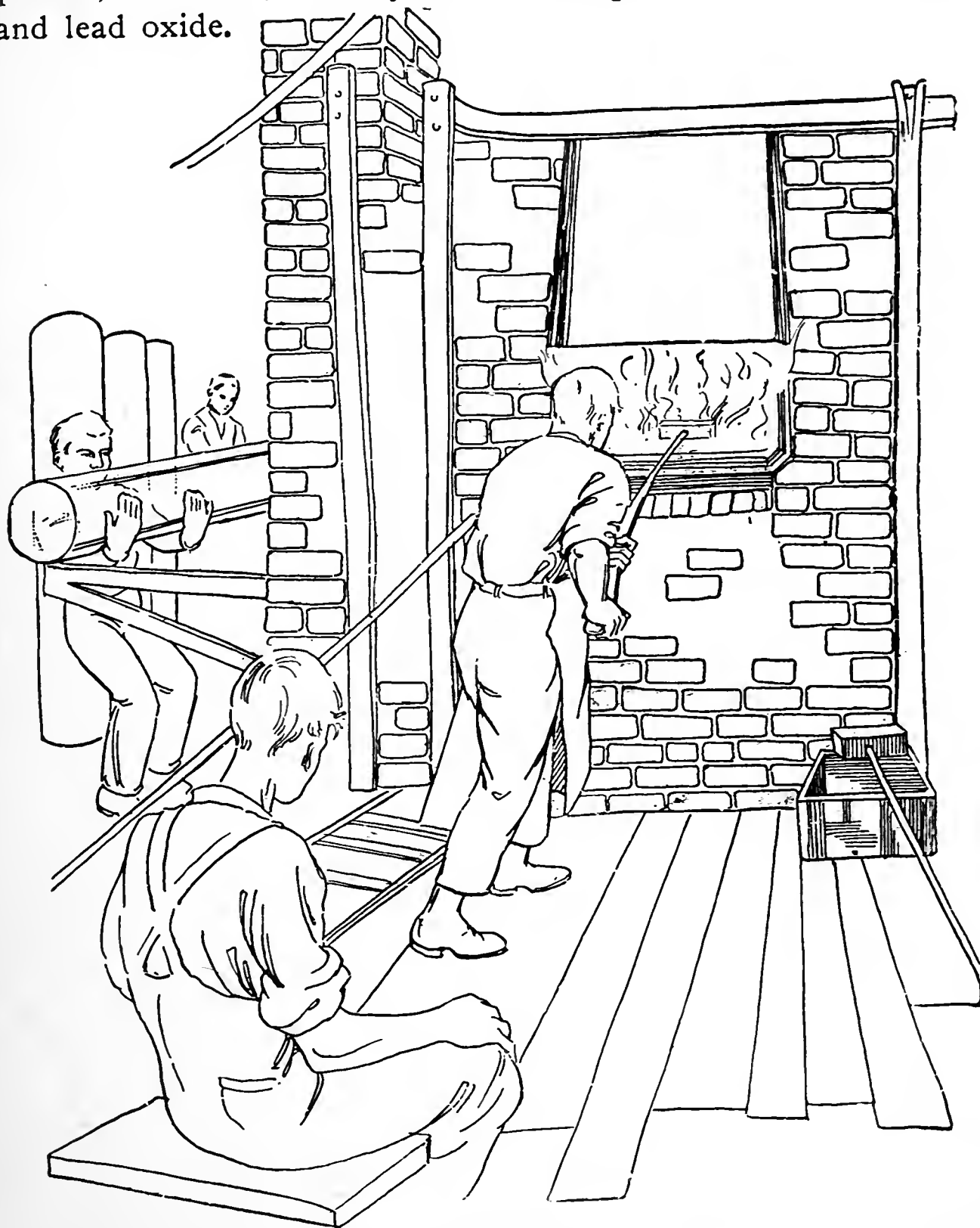
FIG. 22 IRONING THE CYLINDERS FLAT
