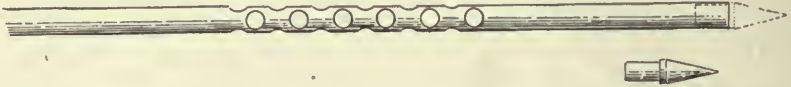
Fig. 186.—Brass tube ( 7\frac{1}{2} inches long and \frac{1}{4} inch in diameter) with (separable) spear point to be passed through the chest for recording lung volume changes. The holes cover a space about 2\frac{1}{2} inches long.
