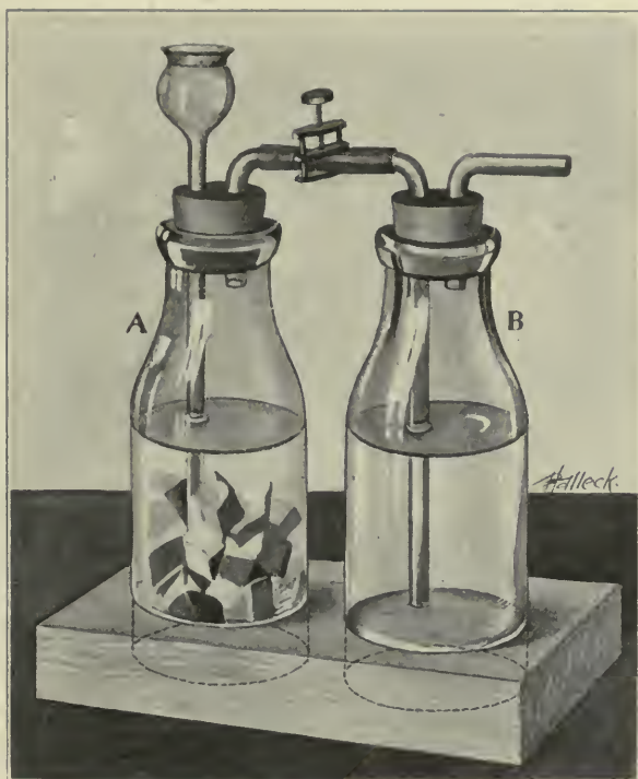
Fig. 114.—Guthrie's carbon dioxide generator. Two quart milk bottles are used to hold blocks of marble and dilute acid (A) and the wash water (bottle B).
