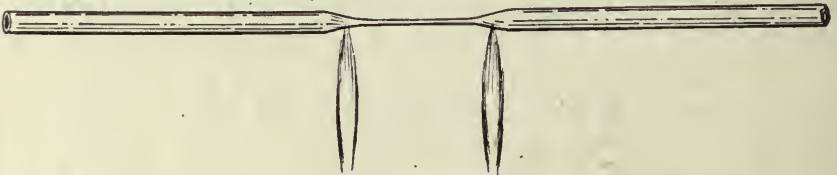
Fig. 379.—The "shoulders" of the cannulas are carefully heated in a needle-pointed flame and drawn out a little to form the "necks" on the two cannulas.
