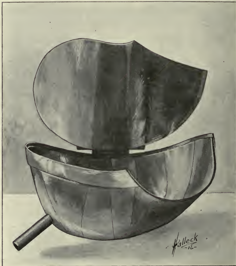
Fig. 338.—Liver oncometer, for the left lobe of the liver of a dog. Made of crimped sheet brass. The lid (raised up) is slipped under the lobe and the cup-like part closes over the lobe to inclose it. The “pedicle” of the lobe passes through the large notch at the right in the picture. The spout is connected to a tambour and the abdomen is closed air tight.
