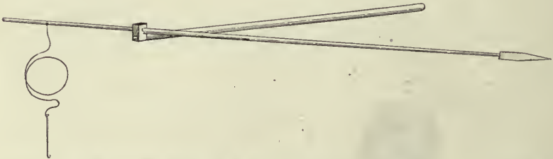
Fig. 62.—Heart lever. The rod is made of 3/16 inch round brass rod into the end of which a small hole is drilled. A small block of wood fiber or hard rubber is attached to the rod by a small wire nail which passes (loosely) through the wood fiber block and is then driven (tightly) into the hole in the end of the rod. The writing lever is a very thin strip split from a long (10 or 12 inches) section of a bamboo fishing pole. This lever, which is very light and limber, passes (tightly) through an oblong hole in the upper part of the wood fiber block. A paper or celluloid (used photographic film) writing point is attached by mucilage or by a cement made by dissolving a photographic film in acetone. These levers are entirely satisfactory for the hearts of frogs, turtles, for uterine strips, etc. They can be made easily and cheaply.
