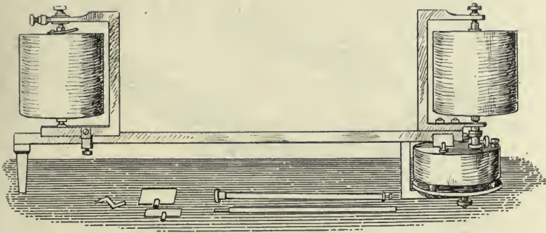
Fig. 26.—Harvard long paper kymograph.
