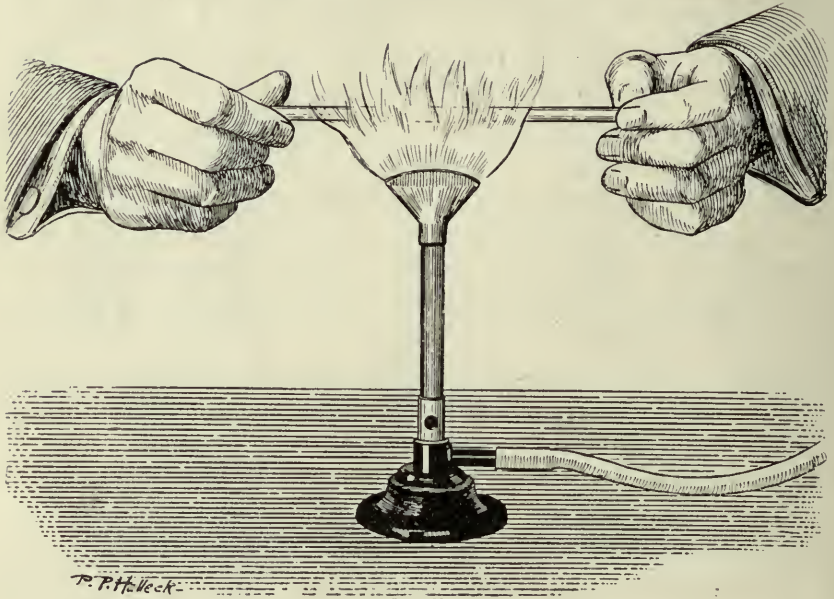
Fig. 381.—Heating a tube before bending. The tube is constantly turned in the fingers.
