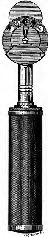
Fig. 163.—Electric ophthalmoscope. The small (replacable) battery is concealed in the handle of the instrument.
