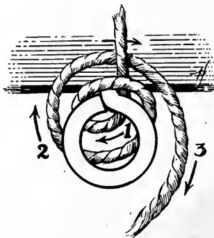
Fig. 81.—Method for quickly fastening the string to the board without tying any knots.
