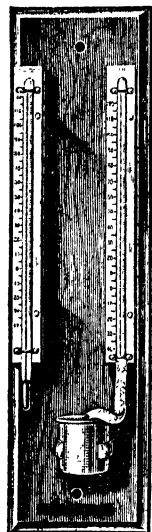
Fig. 64. — Wet- and dry-bulb thermometer.
