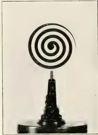
FIG. 12.—Apparatus for producing an after-image of motion, in direction the reverse of the original movement.
