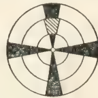
FIG. 6.—Disk for the measurement of the contrast effect in Fig. 5. The cross-hatched segment represents red, which may be varied in amount until the middle zone on rapid rotation matches the middle zone of Fig. 5.
