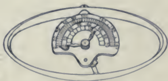
FIG. 26.—Hand dynamometer (Zimmermann, Mk. 27.50; Collin, Fr. 35; Verdin, Fr. 25). The instrument has two kg. scales, an inner scale for squeeze, and an outer scale for pull.—A dynamograph is sold by Verdin for Fr. 130.
