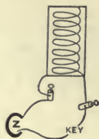
FIG. 16. — Arrangement of inductorium for single (unmodified) shocks. A. Waller, An Introduction to Human Physiology , 1891, 315. Cf. Fig. 11.
