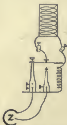
FIG. 11. — Shows the arrangement of the inductorium for (ordinary) repeated shocks. See A. Waller, An Introduction to Human Physiol. , 1891, 315; and cf. Fig. 16.
