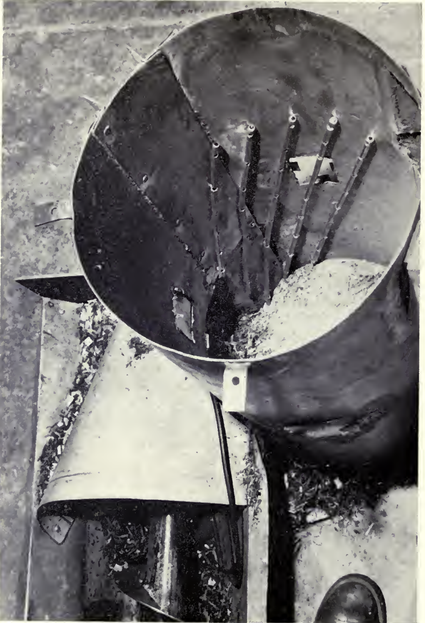
View from top of vertical auger housing with five 5/16-inch rods installed 2 inches apart. Auger rotated clockwise. Inlet opening is on left, outlet on right. (Fig. 6)
