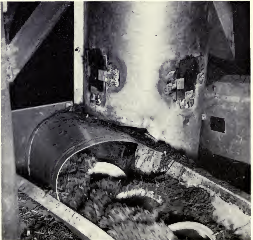
Grass silage moving from 6-inch charging auger to 12-inch vertical auger. (Fig. 9)
