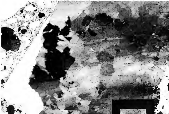
Undulose Extinction within Coarse Aggregate 25x Crossed Polars
