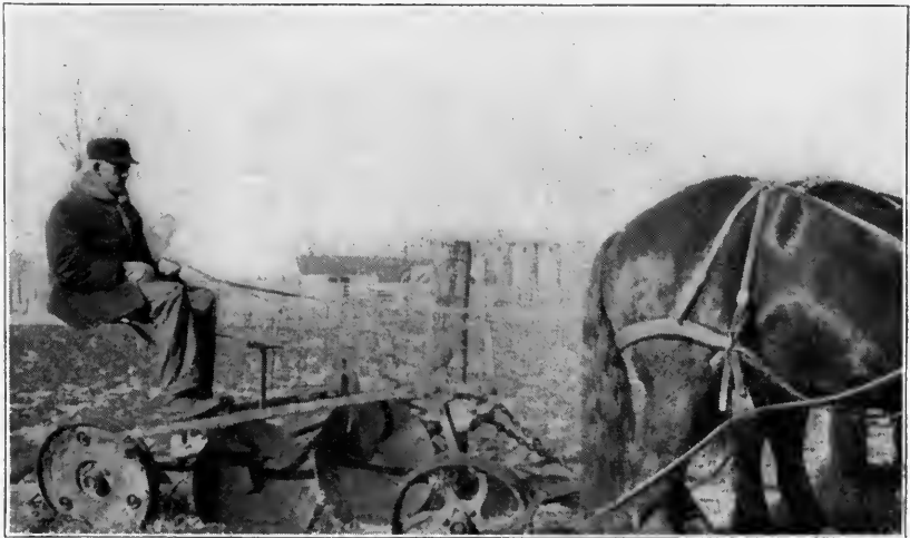
FIG. 3.—DEEP TILLAGE MACHINE. REAR DISK TURNS THE SOIL IN THE BOTTOM OF FURROW MADE BY FRONT DISK
