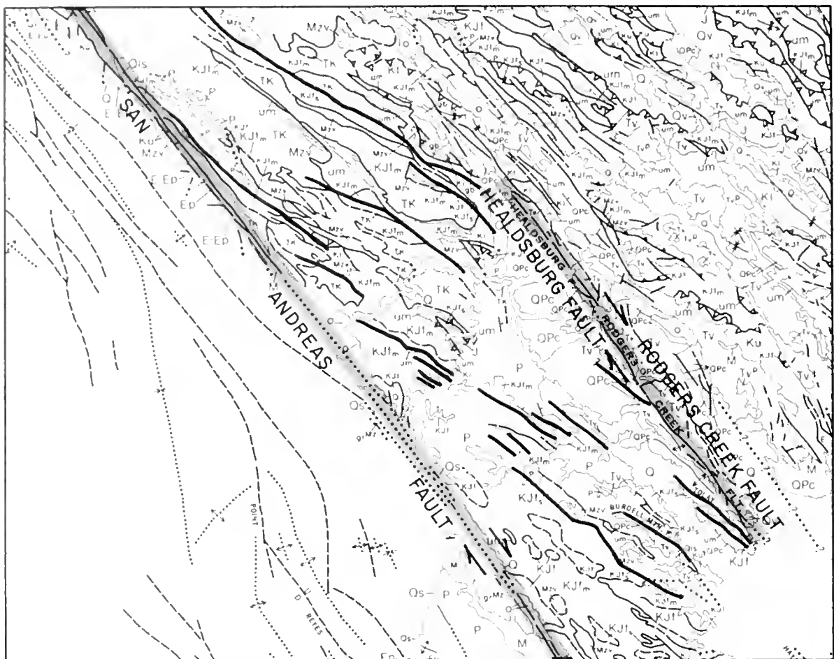
Figure 8. Diagonal faults formed between two major strike-slip faults, the San Andreas and the Rodgers Creek-Healdsburg faults.
