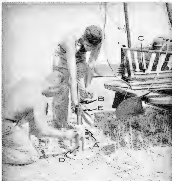
FIG. 317.—Removing steel electrodes after completing electrical measurements. A, hollow-stem hydraulic jack; B, electrode; C, spare electrodes; D, plunger pump; E, electrode clamp. (Courtesy of Union Oil Company of California.)
