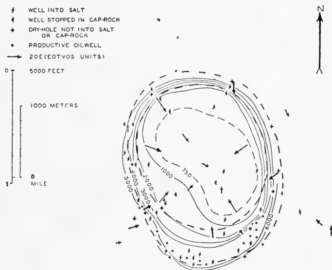
FIG. 210.—Gravity maximum over a shallow salt dome (Nash dome) located in the Gulf Coast, Brazoria and Fort Bend Counties, Texas. (Barton, A.I.M.E. Geophysical Prospecting , 1929.)
