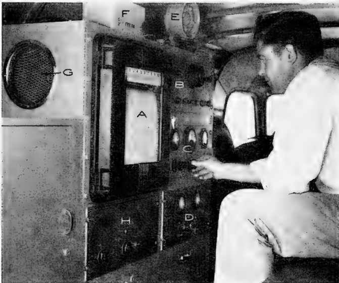
FIG. 686.—Radioactivity logging instrument truck. A, graphic recorder; B, oscilloscope panel; C, amplifier panel; D, power supply panel; E, inter-communicating loudspeaker to hoist operator; F, depth indicating odometer; G, ventilator; H, recorder control panel. (Courtesy of Lane-Wells Company.)
