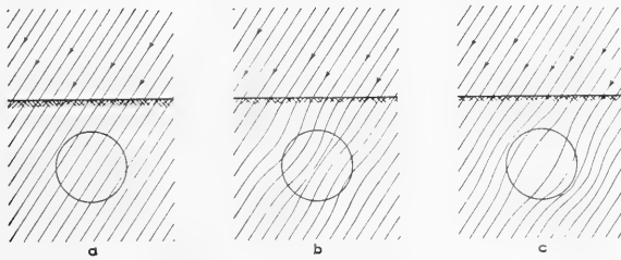
FIG. 13.—Distortion of earth's field due to various materials: (a) non-magnetic material; (b) paramagnetic or ferromagnetic material having a susceptibility greater than the surrounding medium; (c) diamagnetic material, with a susceptibility less than the surrounding medium.
