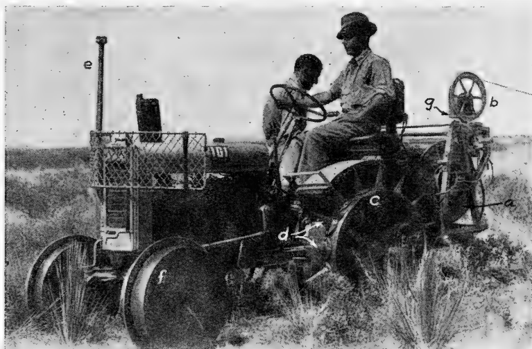
FIG. 318.—Continuous mobile electrode. a , reel of flexible insulated wire; b , measuring sheave wheel; c , steel tractor wheel; d , steel contact stakes; e , guide for reeling-in cable; f , weighted flanged wheels; g , contact ring which actuates measuring signal system. (Courtesy of International Geophysics, Inc.)
