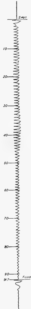
FIG. 701.—Typical reflection record without filter showing shot-point, tubing-collar reflections, and fluid reflections.
