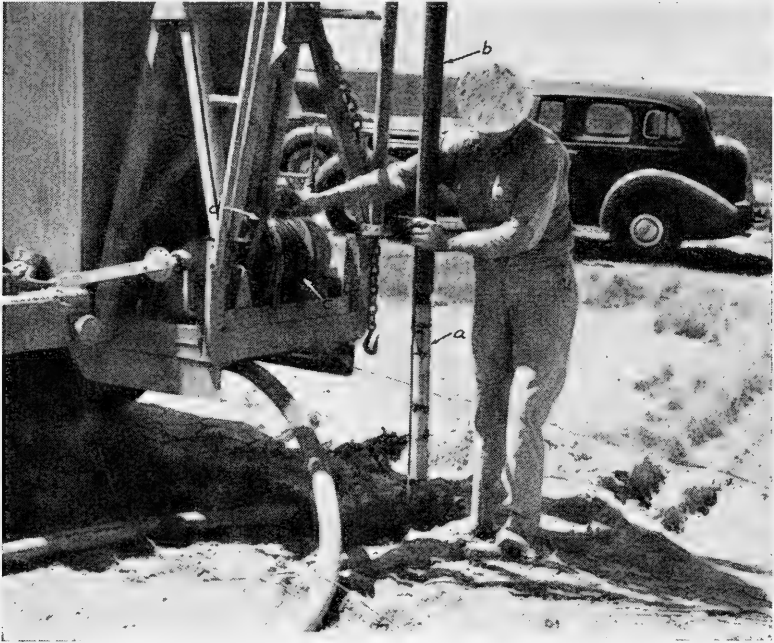
FIG. 542.—Loading deep seismic holes by use of weighted winch lines. a , explosive cartridge; b , weighted tube; c , winch; d , hand control on winch. (Courtesy of United Geophysical Company.)
