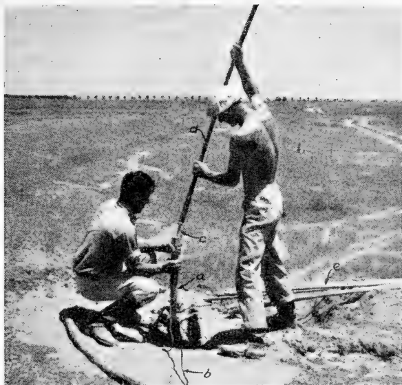
FIG. 540. — Method of loading explosives in a medium depth hole for seismic work. a , explosive cartridge; b , firing wires; c , spear or "schnozzle"; d , loading pole; e , extensions with link couplings. (Courtesy of United Geophysical Company.)
