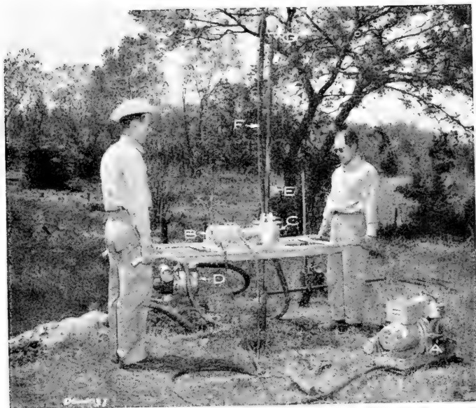
FIG. 556.—Portable drill with gasoline-electric motor drive to rotary table. A, gasoline engine direct-connected to generator; B, electric motor driving rotary table; C, rotary table; D, gasoline engine direct-connected to mud pump; E, Kelly; F, mud hose; G, swivel. (Courtesy of Seismograph Service Corporation.)
