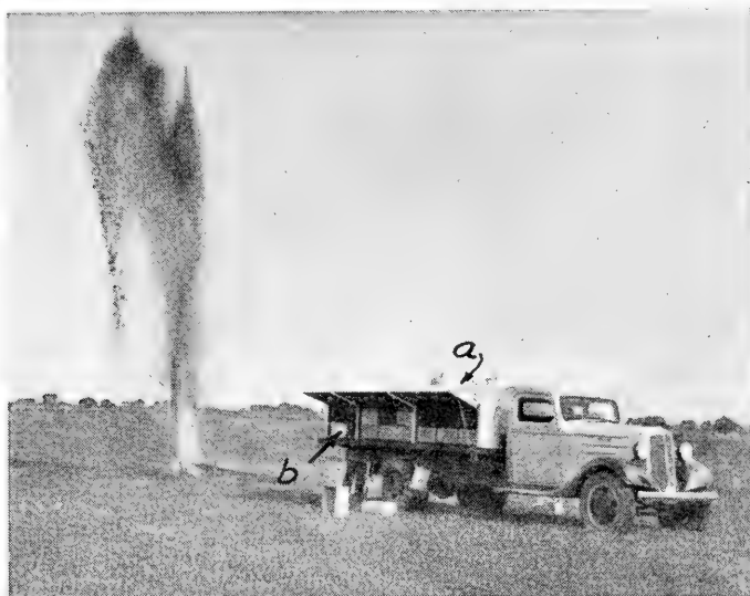
FIG. 543.—Shooting truck and shot-point geyser. a , water tank; b , explosive compartments.
