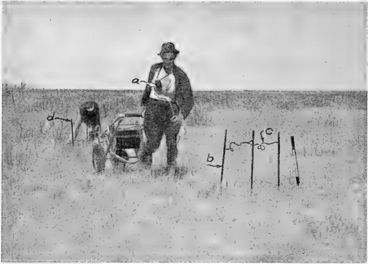
FIG. 323.—Mobile reel in operation. a , small portable telephone; b , steel electrodes; c , flexible connectors; d , previously used set of electrodes. (Courtesy of International Geophysics, Inc.)
