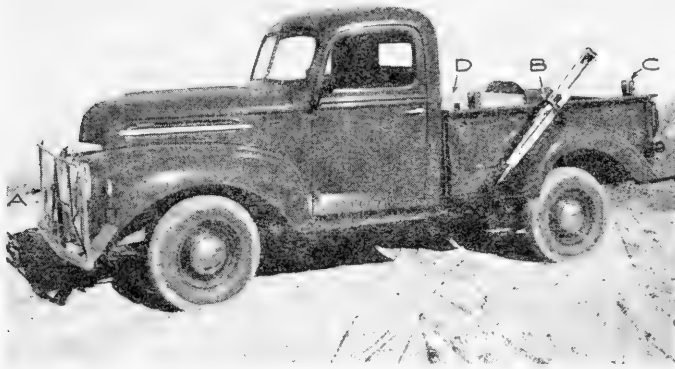
FIG. 526.—Survey pick-up truck. A, brush guard; B, support for transit and alidade tripods; C, "U" supports for stadia rods; D, steel box with lock for storage of surveying instruments. (Courtesy of Griffin Tank and Welding Service.)
