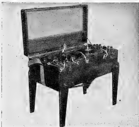
FIG. 325.—Simple millivolt-milliamperere apparatus for resistivity measurements. a , potentiometer battery adjustment; b , high resistance galvanometer; c , ground current neutralizer; d , potentiometer dial; e , 0-10 milliamperere meter; f , range switch for milliammeter giving values to 2000 milliampereres; g , galvanometer shunt and potentiometer switch keys.
