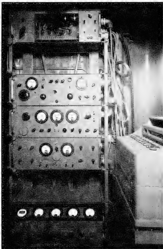
FIG. 667.—Control panels and recording camera for electrical logging of oil wells. (Courtesy of Schlumberger Oil Well Surveying Company.)
