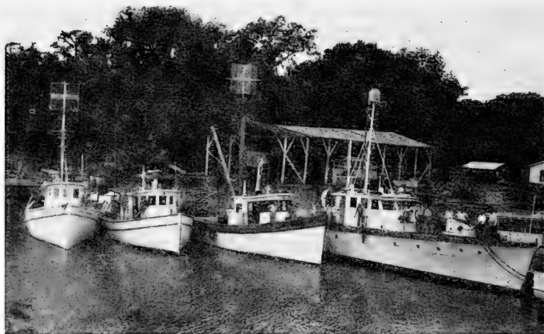
FIG. 568.—A marine seismic fleet consisting of two survey boats, a shooting boat and a recording boat. These boats are (SF-1) fadar-equipped; note radar antennae and reflectors. (Courtesy of American Exploration Company.)
