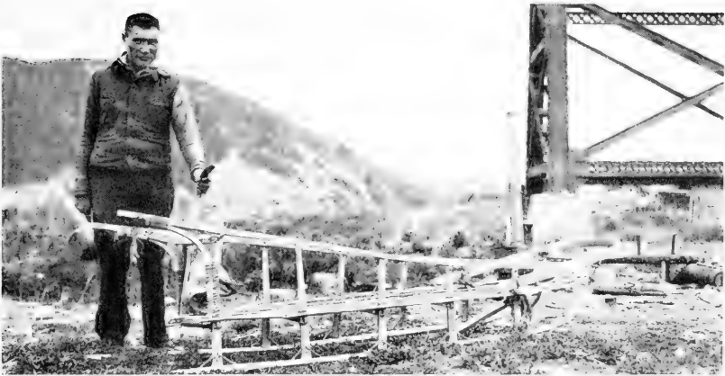
FIG. 154.—Chief Thomas of Nenana, Alaska, with his sled which is fastened together with sinew.
