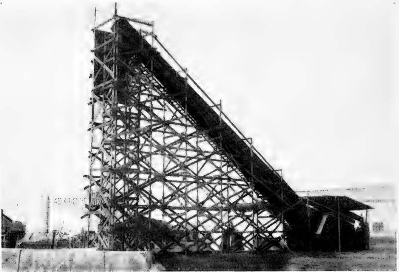
FIG. 62.—The astronomical camera, so large that two operators sat inside to change the plates during the eclipse. (Photograph by Kellers.)
