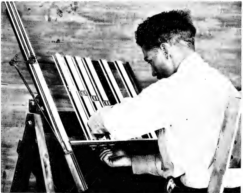
FIG. 5.—Field-director Freeman reducing observations with our slide-rule machine, which saves three-fourths the computing.
