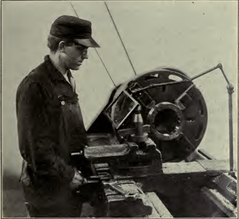
Fig. 7.—Glass chip-shield on lathe. Shield is supported by a universal jointed arm secured to tool carriage, so that it can be readily adjusted. United States Steel Corporation.
