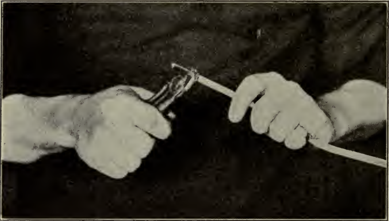
Fig. 37.—Crimping detonator on fuse. United States Bureau of Mines.
