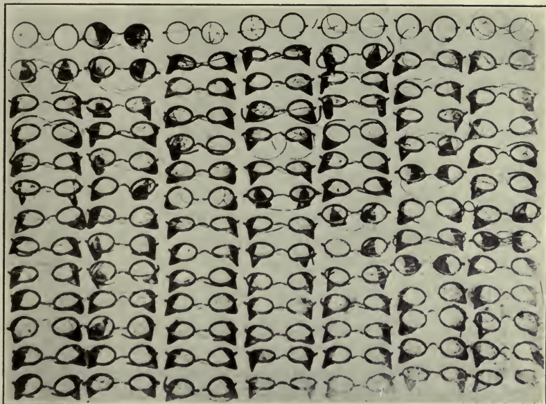
Fig. 38.—Ninety-four pairs of broken goggles collected in three months. Each pair saved a man's sight. American Steel Foundries.
