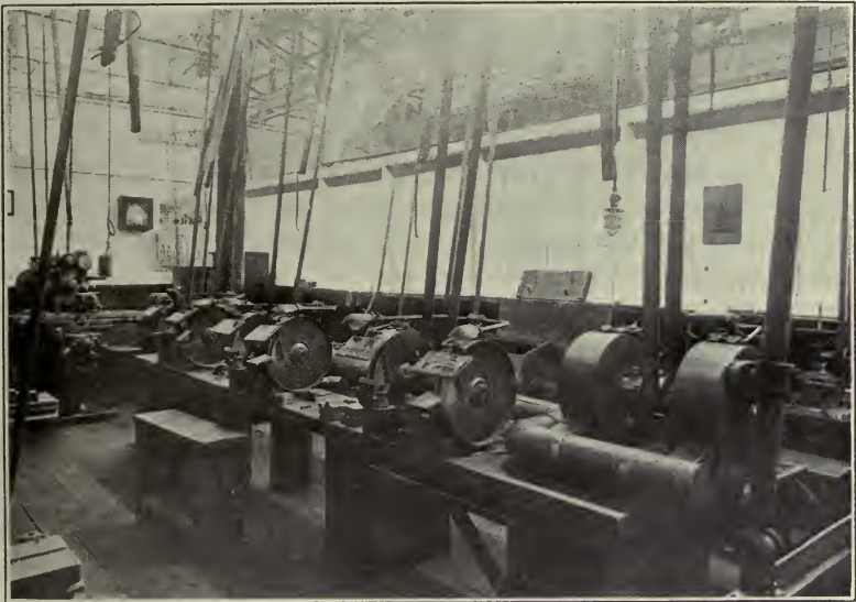
Fig. 10.—Motor-driven emery wheels, equipped with plate-glass shields, hoods, and exhaust system for removal of dust. United States Steel Corporation.
