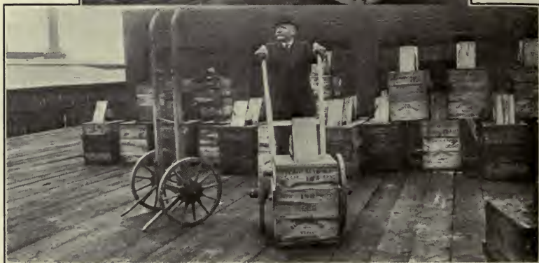
Fig. 32.—One-man truck for 18-inch carboy, with detachable adjustment for handling lead carboys. A safe, light, smooth-running, and inexpensive carrier. General Chemical Company.
