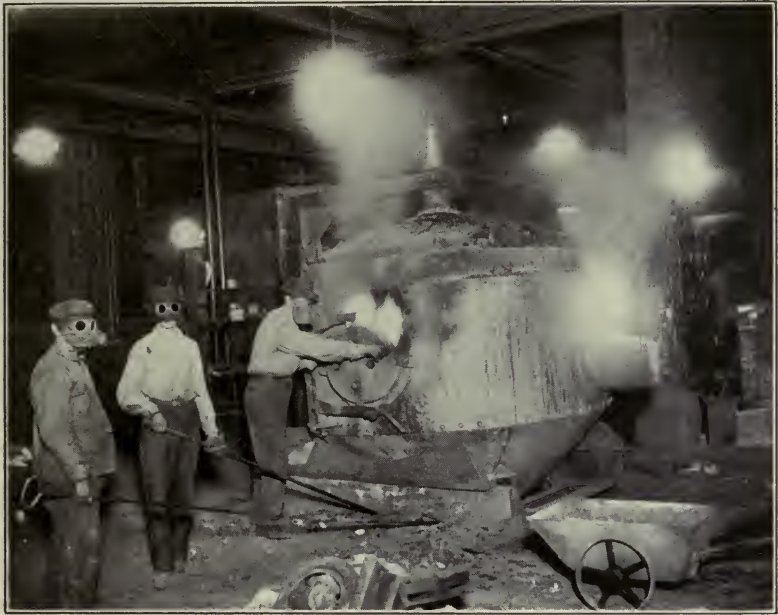
Fig. 23.—Operatives wearing masks and goggles for protection from intense light and heat. Otis Elevator Company.
