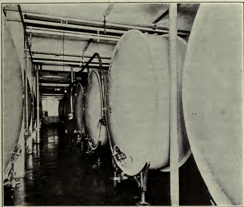
Fig. 36.—Glass-lined steel vats, which do not require varnishing.
