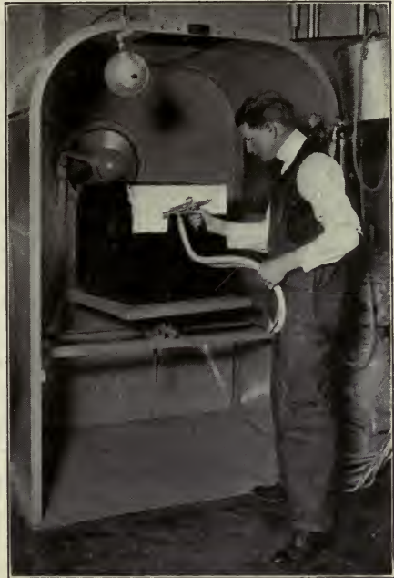
Fig. 34.—Applying a finish by the spray process, showing hood and exhaust for removal of noxious fumes. American Museum of Safety.
