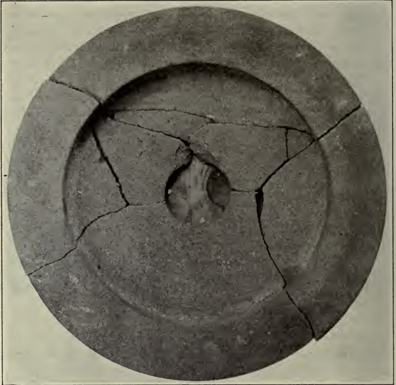
Fig. 9.—A serious or fatal accident from the breaking of this wheel was prevented by the hood which inclosed it. Oliver Mining Company.
