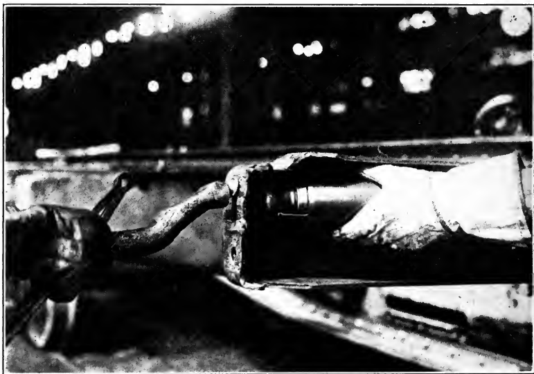
Fig. 15.—Unsafe practice of only partially covering rivet head with dolly-bar. Haskell and Barker Car Company.
