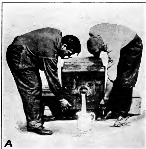
Fig. 30.—The handling of acids ( A , Unsafe and inefficient method). Horace M. McCord & Co.
