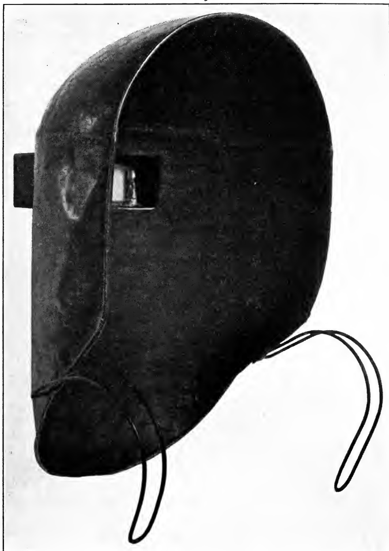
Fig. 18.—Mask used by electric welders and scrap burners. Made of sheet brass and goggles. Weight is carried on shoulders by means of the wire stirrup. National Tube Company.
