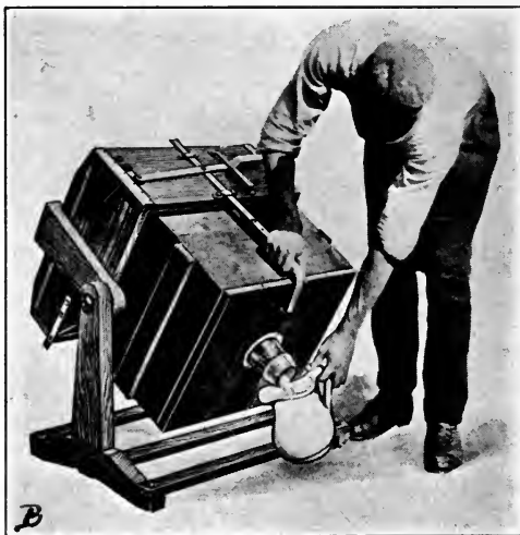
Fig. 31.—The handling of acids ( B , Safe and efficient method). Horace M. McCord & Co.
