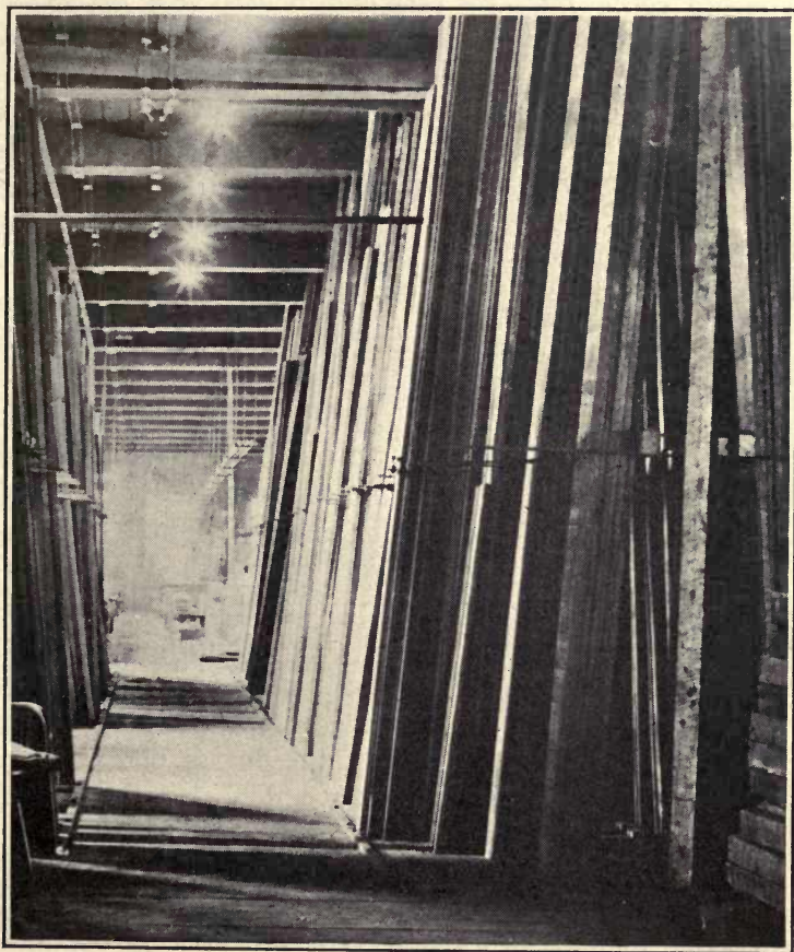
FIG. 28.—Vertical stowage of lumber in sizes up to 2 by 12 in. by 16 ft.
