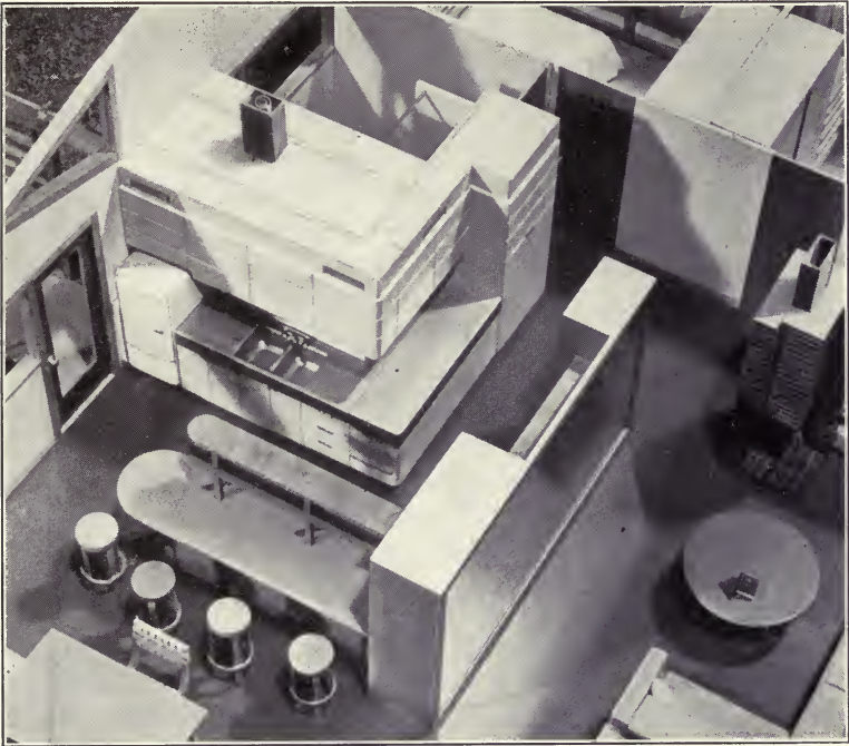
Figure 111. Model display of house equipped with prefabricated heating and utility unit (upper left).
