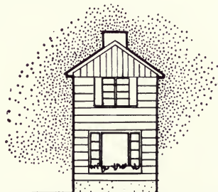
CHIMNEY ENLARGED, WIDE SIDING MATERIAL ADDED; EAVES SHORTENED
