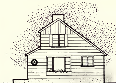
EAVE LINE LOWERED OVER ADDITION
