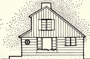
WALL MATERIAL CHANGED ABOVE WINDOW HEAD
