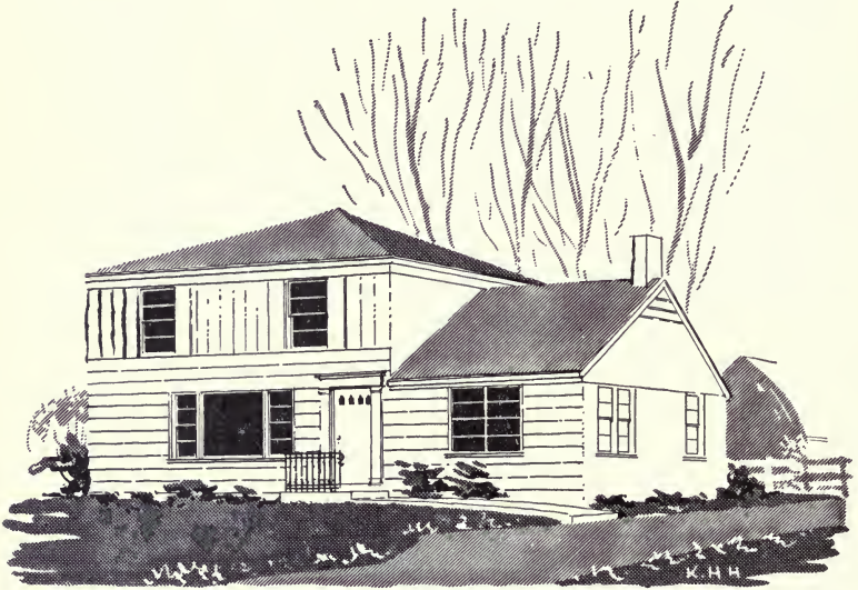
Figure 86. Remodeled exterior of square two-story house with one-story wing. See Figure 6 for original.
