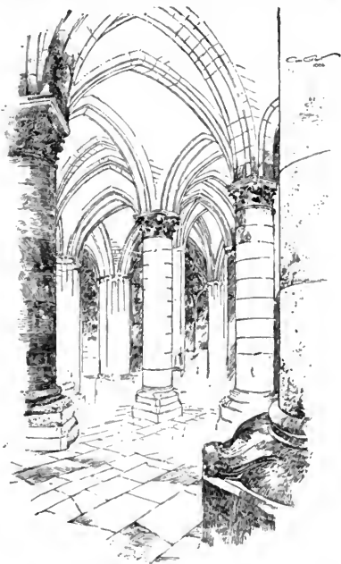
Fig. 63. Perspective of vaulting as applied in a double curved apsidal aisle, Notre Dame, Paris.
