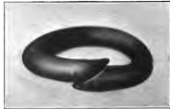
FIG. 37. SHOWING SCARFS ON LAP WELD OF RING.
