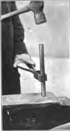
FIG. 12. SQUARING AN END, ALSO UPSETTING.
