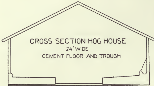
FIG. 389. CONCRETE FLOOR FOR HOGHOUSE.
