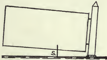
FIG. 508. HOW A GATE IS HUNG.
