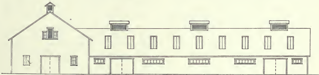
FIG. 230. A HYGIENIC DAIRY BARN (SIDE ELEVATION).
