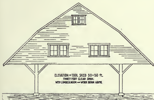
FIG. 424. TOOLHOUSE AND WORKSHOP (ELEVATION).
