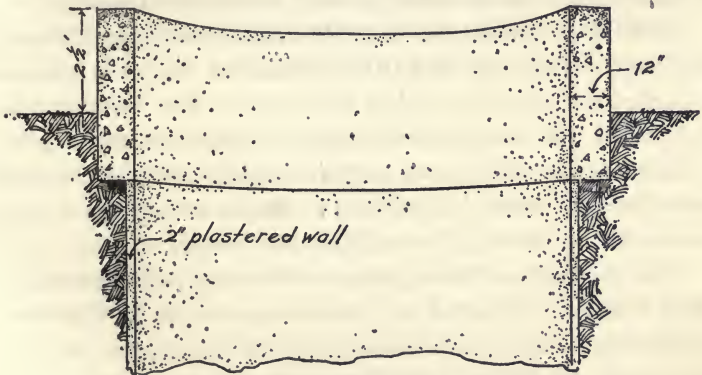
FIG. 78. — Construction of Pit Silo.
