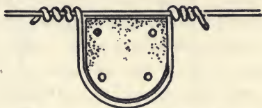
FIG. 57. — Attachment of Wire to Post.
