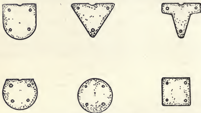
FIG. 55.— Cross Sections of Different Shapes of Posts.
