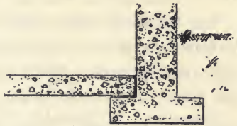
FIG. 26. — Waterproof Joint between Footing and Floor.
