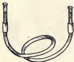
FIG. 25. — Simple Level Made of Hose and Glass Tubing.
