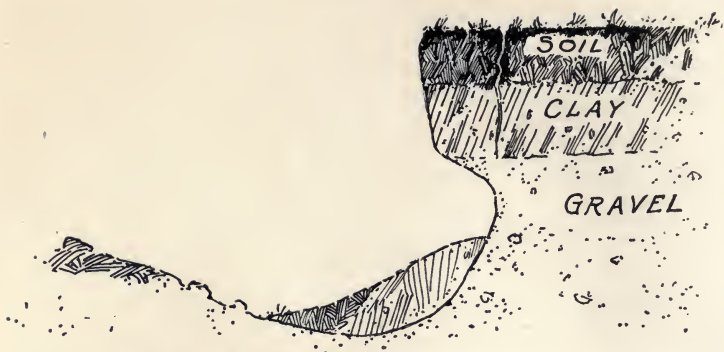
FIG. 6. — What Actually Happens in Removing Gravel from Small Pits.
