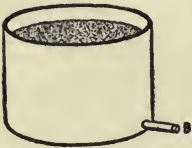
Figure 28. Pot of soil from which the capillary moisture has been dried out by exposing it for some weeks to the air, followed by several days of baking in an oven sufficiently hot to turn all moisture to steam, and thus driving it out leave the soil dry of water, water free, "dry substance," as when pot 1, Figure 20, of baked soil was first placed in the air.
