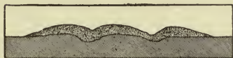
Figure 180. Roadway made of 8 inches of gravel on peat, which the wheels soon punch into the soft muck.
