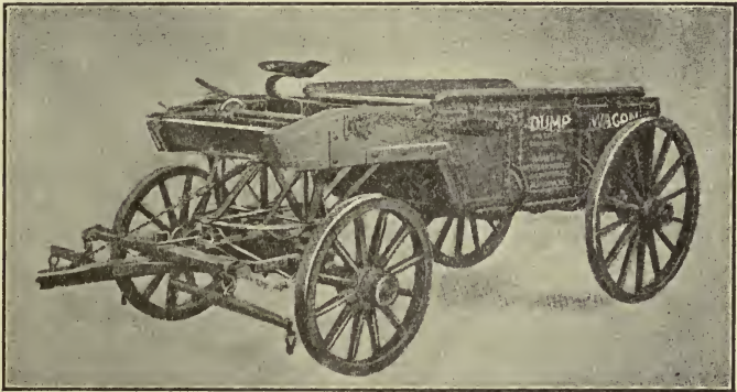
Figure 210. Dump wagon, with lever and chain gear to open and close drop bottom.
