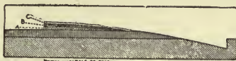
Figure 179. Cross-section of macadam road. A, lower layer of 6 or more inches of 2 to 3-inch stone; B, middle layer of 1 to 2-inch stone; C, layer of broken stone under 1 inch, dust, etc.
