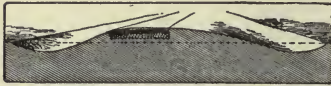
Figure 219. Macadam road on one side of the center of the grade and an earth track on the other side.
