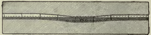
Figure 102. Quiet water in a sag in a drain tile allows sediment to settle there and clog the drain.
