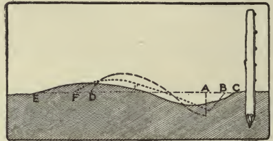
Figure 182. In throwing earth from roadside ditch to the center of the roadway with the reversible road machine the operator can make a ditch with vertical outer bank, leaving the ditch and earth as shown by the line A D; slanting outer banks, as at B F; or rounded bank, as at C E.
