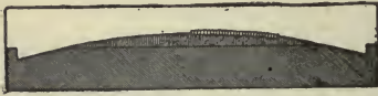
Figure 229. Road with track 9 feet wide one side of the center laid with brick. Below the brick there must be a layer of gravel or other solid material several inches deep, as when wet bricks are crushed into a clay bed by the wheels of heavy vehicles.
