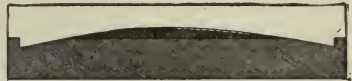
Figure 230. Roadway covered 8 to 12 feet wide with granite blocks, very hard sandstone or blocks made of sand and cement, about 4 x 6 x 12 inches, with 6 x 12-inch surface up, laid on a layer of gravel or sand.
