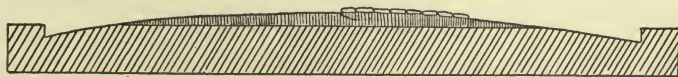
Figure 232. Roadway paved with cobblestones laid on gravel makes a very rough, but very durable, hard roadway.
