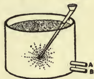
Figure 29. Pot of air-dry soil, containing only hygroscopic water. Through the funnel tube water is slowly run into the center of the mass of soil. The water is carried away from the point of the tube in all directions by the force of capillarity. Gravity causes a slight tendency for more to go downward than in other directions. But capillarity, being much the more powerful acting force under these conditions, causes the water to go upward and side-wise as well as downward.
