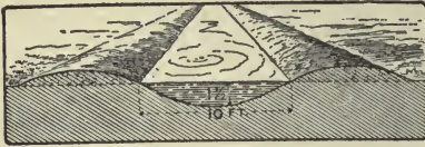
Figure 156. Supply ditch as made with reversible road machine or with plow and scraper, as in Figures 117 and 155.
