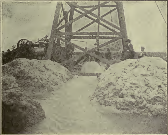
Figure 139. Portable engine used for pumping water for flooding rice fields in Texas.
