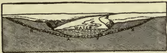
Figure 239. Cross-section of a ford across a creek. Ordinary water level in a stream shown. The dotted lines represent ford graded down and surfaced with stone. In many instances the bed of the stream is solid and the stone surfacing is necessary only at the outer edge of the water, as at R-A or X-Y.
