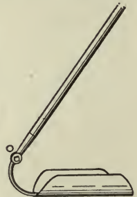
Figure 92a. Tile hoe, adjustable to push or pull.
