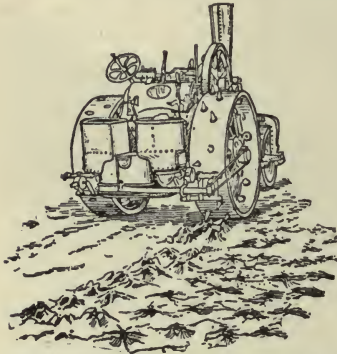
Figure 236. Steam road roller. Spikes in wheel used to break up macadam surface that the broken stone may be remixed, rolled and resurfaced.
