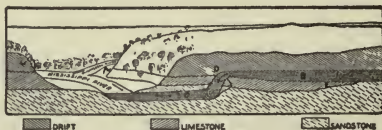
Figure 12. The Falls of St. Anthony when its recession had just begun. A, water in the Minnesota, after it had ceased to receive the glacial water. B, water in the Mississippi river above the falls. C, water in the Mississippi river below the falls. D, the Falls of St. Anthony when yet at a point near the confluence of the two rivers.
