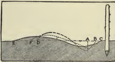
Figure 118. Showing forms of ditch beside a fence line, as at the side of a public highway. A-D, ditch made with steep bank and dirt left in high ridge. B-F, ditch made with slanting outer bank and ridge rounded down. C-E, ditch rounded and earth spread out so that land can be mowed or even cultivated to the roadway, as at P.
