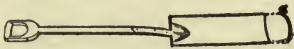
Figure 90. Tile or ditching spade, blades made 18, 20 and 22 inches long, 6 to 7 inches wide, and much curved, as shown in cross section at A. This is a surprisingly useful tool in opening tile or open drains in many easily worked soils. By turning it at an angle as shown in Figure 93 the bottom of the ditch may be made as narrow as desired for a 3 or 4-inch tile.
