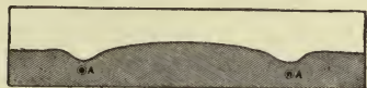
Figure 193. Line of drain tile, laid 1 to 3 feet deep, under each side of roadway.
