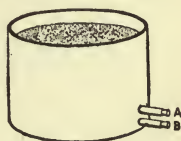
Figure 21. Pot of baked soil after standing several days in the air, when it weighs a few pounds more from the absorption of "hygroscopic" moisture.
