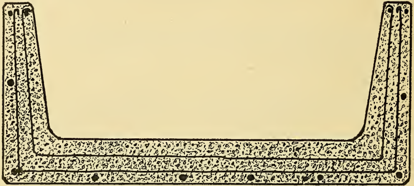
Plate 36. Cross section of a watering trough showing, "a", sloping internal side walls; "b", filleted or rounded corners or angles; "c", the placing of reinforcing wires. The large dots represent the ends of the side and bottom wires. The position of the wires which reach from the top at one side around the bottom and up to the top at the other side, is also shown.
