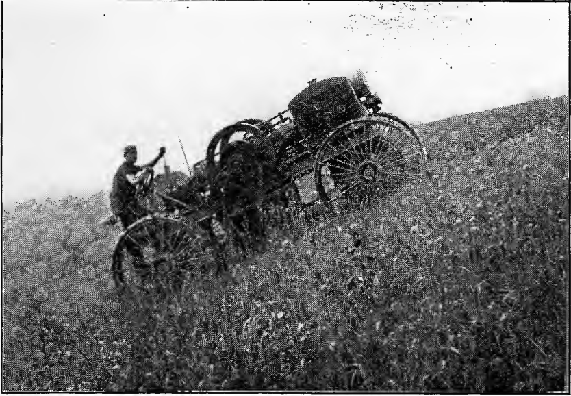
Plate 3. "Four-wheeled drive" tractor ascending 64 per cent. grade. In general, tractors have little difficulty in climbing a steep hill which affords a good foothold or grip.
