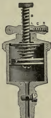
SECTIONAL VIEW IDEAL GREASE CUP.
