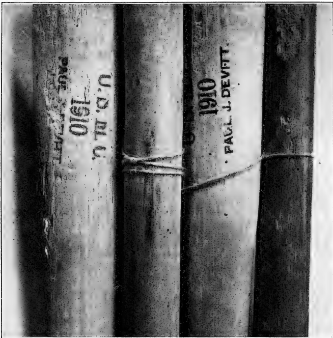
FIG. 3.—Powder-posted hickory pickaxe handles, showing exit holes of adult beetles; work of Lyctus linearis . (Original.)
