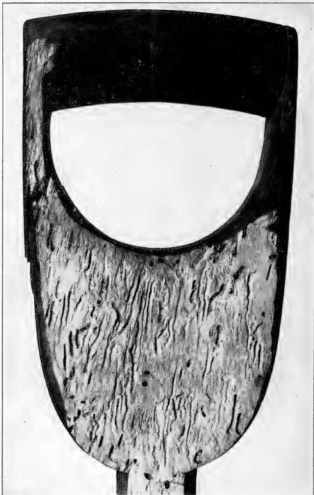
FIG. 2.—Powder-posted ash shovel handle with surface wood cut away to show burrows of larvæ within; work of Lyctus planicollis . (Snyder.)
