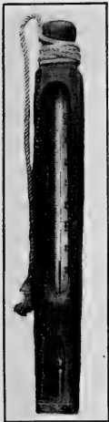
FIG. 14.—Thermometer used by Bureau of Animal Industry inspectors, in holder whitened from a block of wood.
