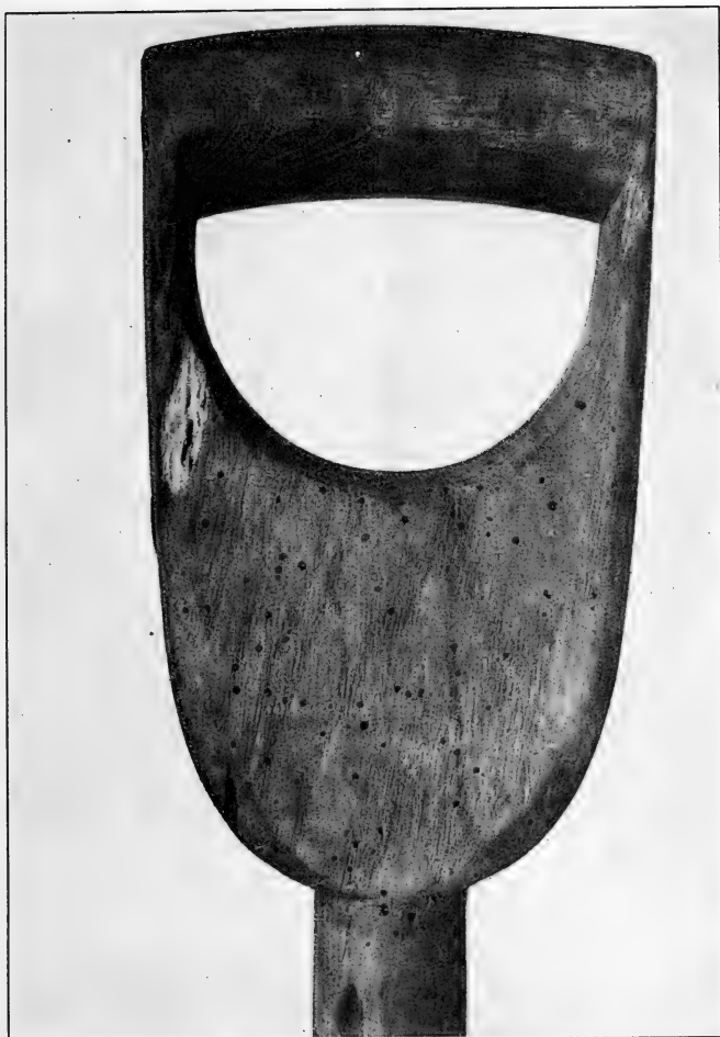
FIG. 1.—Powder-posted ash shovel handle, showing exit holes of adult beetles; the work of Lyctus planicollis . (Original.)
