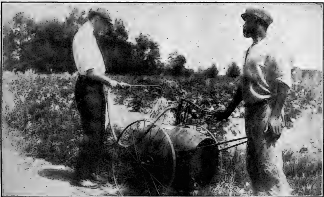
FIG. 8.—Portable barrel pump for application of herbicide to weed borders.
