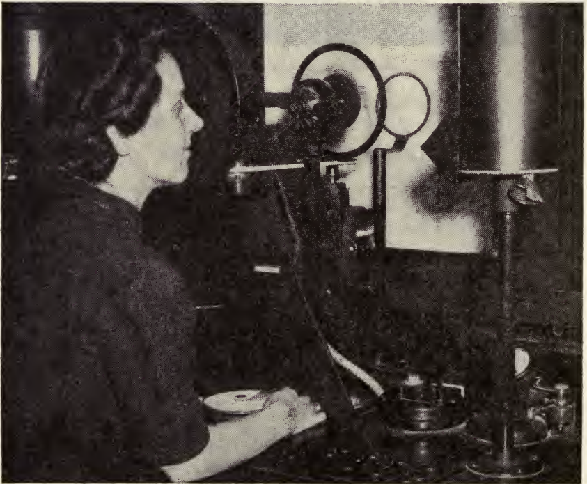
Figure 5.—Using a specially constructed precision instrument, a worker measures the color of cotton. Color measurement is an aid in the preparation of standards for farm products.
