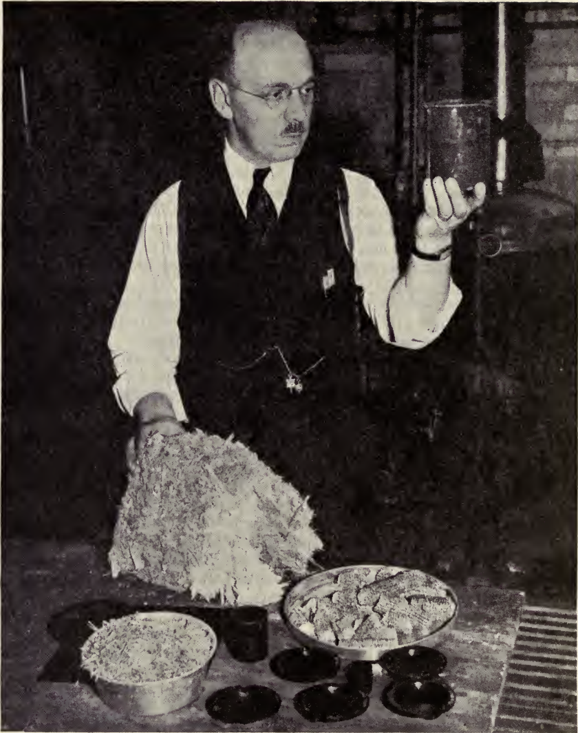
Figure 1.—An example of fundamental research with a practical objective—in this case, the use of byproducts. On the table are sugarcane bagasse, straw (in foreground), and corncobs—possible sources of molding powder like that in the beaker. In the foreground are plastics made from the molding powder.
