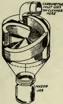
A—A PHANTOM VIEW OF A BENNETT CARBURETOR AIR CLEANER
