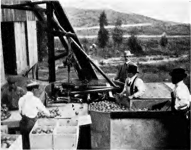
FIG. 124.—Showing the method of washing oranges to remove the sooty mould fungus. (Bulletin No. 123, United States Department of Agriculture, Bureau of Plant Industry.)
