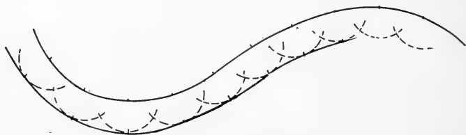
FIG. 129.—A good method for measuring the opposite side of a curved road.
