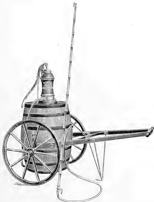
FIG. 58.—A barrel sprayer, mounted on wheels. (Barnes Manufacturing Company.)
