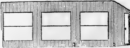
ELEVATION.—LENGTH, 24 FEET; WIDTH, 11 FEET; HEIGHT, IN FRONT, 9 1-2 FEET; HEIGHT, IN REAR, 6 1-2 FEET.
