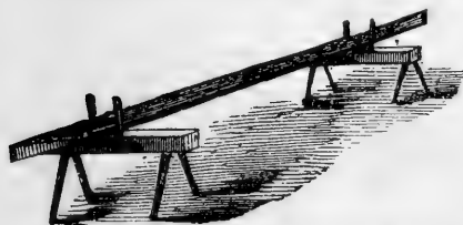
FIG. 3.—TRESTLE FOR POINTING THE RAILS.
