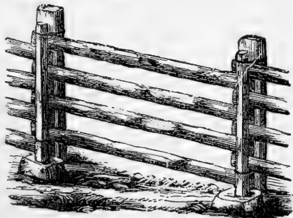
SECTION OF STRAIGHT RAIL FENCE.
