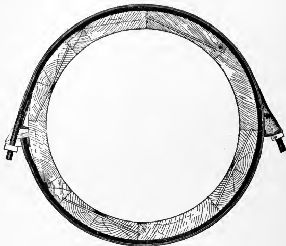
FIG. 27—CROSS-SECTION OF STAVE PIPE.
