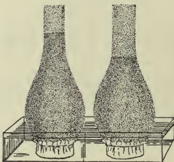
FIG. 35.—Water rises more rapidly by capillarity through fine soils than in coarse soil.
