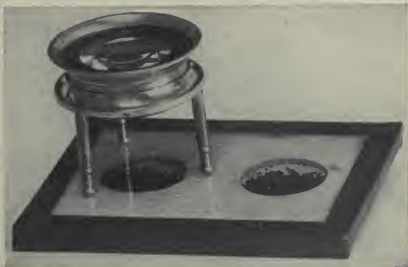
FIG. 11.—Seeds mounted in holes in heavy pasteboard between two pieces of glass held with paper binding. A tripod lens used for seed study. (Agricultural Education.)
