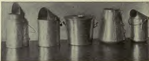
FIG. 216.—Five styles of milk pails, intended to reduce the amount of dirt in milk which falls in from cows and from milkers. Which do you consider the best form for this purpose?
