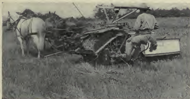
FIG. 84.—A modern grain harvester. All small grains are cut and bound into bundles by this machine. The tying part of the machine is one of the greatest inventions of modern times.
