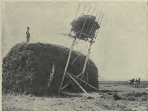
FIG. 58.—Hay-stacking machine. The hay is taken from the sweep rake (Fig. 65) and lifted to the stack by horse-power. Notice the horses at the end of the rope. (Plant Industry.)
