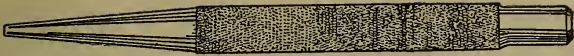
Figure 45.—Nail Set. On all wooden surfaces to be painted nails should be carefully driven with a round peen nail hammer and the heads sunk about one-eighth of an inch deep with a nail set. The holes may then be filled with putty and covered smoothly with paint.
