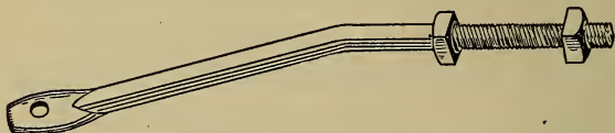
Figure 89.—Wagon-Box Brace. It is offset to hold the rake and to brace the sideboard at the rear and the front ends and sometimes in the middle of light wagon beds.
