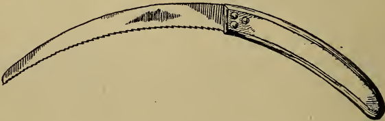
Figure 14.—Bramble Hook for trimming berry bushes and cleaning out fence corners. It has a knife-edge with hooked sawteeth.
