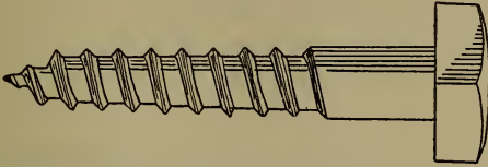
Figure 87.—Lag Screw. To set a lag screw in hardwood, bore a hole the size of the screw shank as calipered between the threads.
