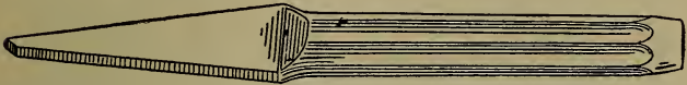
Figure 47.—Cape Cold-Chisel. It may be tapered both ways or one way to a cutting edge, or one edge may be rounded.
