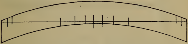
Figure 184.—Diagram showing how to cut a plank on a band-saw to form a curved rafter. The two pieces of the plank are spiked together as shown in the lower drawing. This makes a curved rafter without waste of material.
