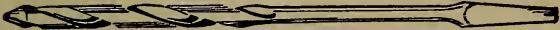
Figure 25.—Wood-Boring Twist Drill Bit. Twist drills for wood have longer points than drills for boring iron.
