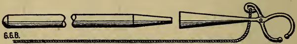
Figure 232.—Hog Catching Hook. The wooden handle fits loosely into the iron socket. As soon as the hog's hind leg is engaged the wooden handle is removed and the rope held taut.
