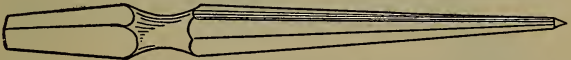
Figure 52.—Taper Reamer. Used to enlarge, or true, or taper a hole that has been drilled or punched.
