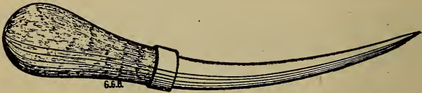
Figure 207.—Marline Spike. Used for splicing ropes, tying rose knots, etc.
