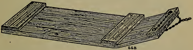
Figure 158.—Stone-Boat. Stump logs are selected for the planks. The bend of the planks is the natural curve of the large roots. The sawing is done by band saw cutting from two directions.
