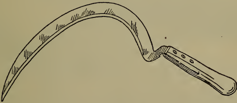
Figure 143.—Grass Hook, for working around borders where the lawn-mower is too clumsy.
