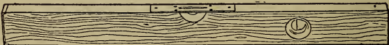
Figure 23.—Carpenter's Level. For practical farm work the level should be 24" or 30" long. Wood is the most satisfactory material. The best levels are made up of different layers of wood glued together to prevent warping or twisting. For this reason a good level should be carefully laid away in a dry place immediately after using.
