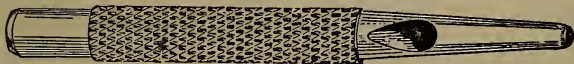
Figure 204.—Belt Punch. Two or three sizes should be kept in the tool box. Belt holes should be small to hold the lace tight. The smooth running of belts depends a good deal on the lacing. Holes punch better against the end of a hickory block or other fine grained hardwood.
