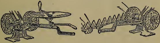
Figure 36.—Emery Grinder. The illustrations show two kinds of grinding that double emery wheels are especially adapted to. To grind a mowing-machine knife it is necessary to reverse. By placing the rest opposite the center between the two wheels the bevel will be the same on both sides, or edges, of the section.
