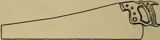
Figure 12.—Hand Saw. This pattern, both for cross cut and rip saw, has been adopted by all makers of fine saws. Nine teeth to the inch is fine enough for most jobs on the farm.
