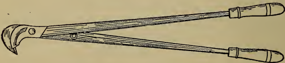
Figure 212.—Tree Pruners. The best made pruners are the cheapest. This long handled pruner is made of fine tool steel from the cutting parts clear to the outer ends of the wooden handles. A positive stop prevents the handles from coming together. Small one-hand pruning nippers are made for clean cutting. The blades of both pruners should work towards the tree trunk so the hook will mash the bark on the discarded portion of the limb.
