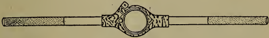
Figure 82.—Stock for Round Dies. The opening is turned true and sized accurately to fit. The screw applies pressure to hold the die by friction.
