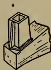
Figure 165.—Hollow Malleable Iron Bolster Stake to hold a higher wooden stake when necessary.
