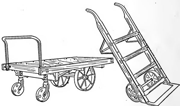
Figure 225.—Barn Trucks. The platform truck is made to move boxed apples and other fruit. The bag truck is well proportioned and strong, but is not full ironed.
