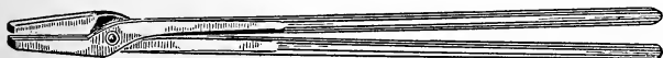
Figure 58.—Blacksmith Tongs. Straight tongs made to hold \frac{3}{8} " iron is the handiest size. Two or three pairs for larger sizes of iron and one pair smaller come in handy.
