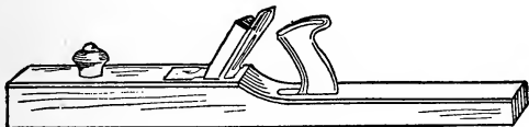
Figure 33.—Fore-Plane. This style plane is preferred to a regular jointer for most farm work.
