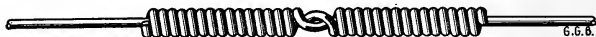
Figure 74.—Wire Splice. With a little practice wire may be wound close enough to prevent slipping.
