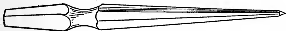
Figure 52.—Taper Reamer. Used to enlarge, or true, or taper a hole that has been drilled or punched.
