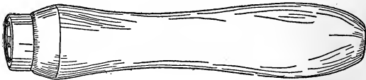
Figure 44.—File Handle. Basswood makes the most satisfactory file handles. They are fitted by carefully turning them onto the file shank to take the right taper. There should be a handle for each file. The handle should be the right size and fitted straight with the file so the file will take the same angle to the work when turned over.
