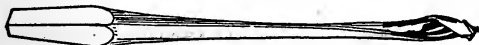
Figure 26.—Pod-Bit. The fastest boring gimlet bits are of this pattern. They are made in sizes from \frac{1}{8} " to \frac{3}{8} " and are intended for boring softwood.
