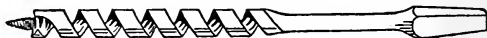
Figure 29.—Ship Auger. This shape auger is made with or without a screw point. It will bore straighter in cross-grained wood without a point.
