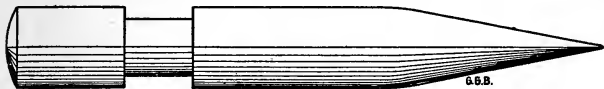
Figure 202.—Husking-Pin. The leather finger ring is looped into the recess in the wooden pin.
