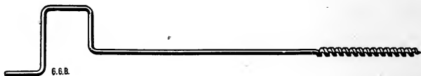
Figure 31.—Bridge Auger. The long handle permits the workman to stand erect while boring. The home made handle is welded onto the shank of a ship auger.
