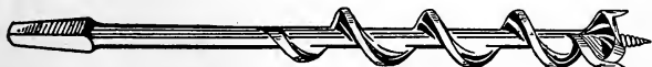
Figure 27.—Auger-Bits. For smooth boring the lip bits are best. The side cutters project beyond the cutting lips to cut the circle ahead of the chips. For boring green wood the single-worm clears better than the double-worm bit.
