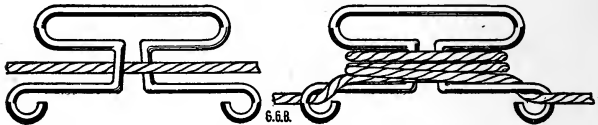
Figure 229.—Clothes Line Tightener. This device is made of No. 9 wire bent as shown in the illustration.
