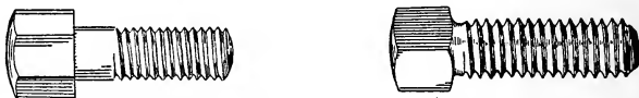
Figure 94.—Machine-Bolt and Set-Screw. The bolt to the left is used to clamp cylinder heads in place. The set-screw to the right is the cup variety. The end is countersunk to form a cup with a sharp rim.
