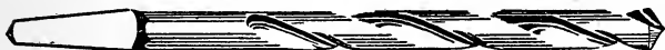
Figure 51.—Twist-Drills. Round shank for the post drill and square taper shank for brace work. Brace drills are small, \frac{1}{4} " or less.
