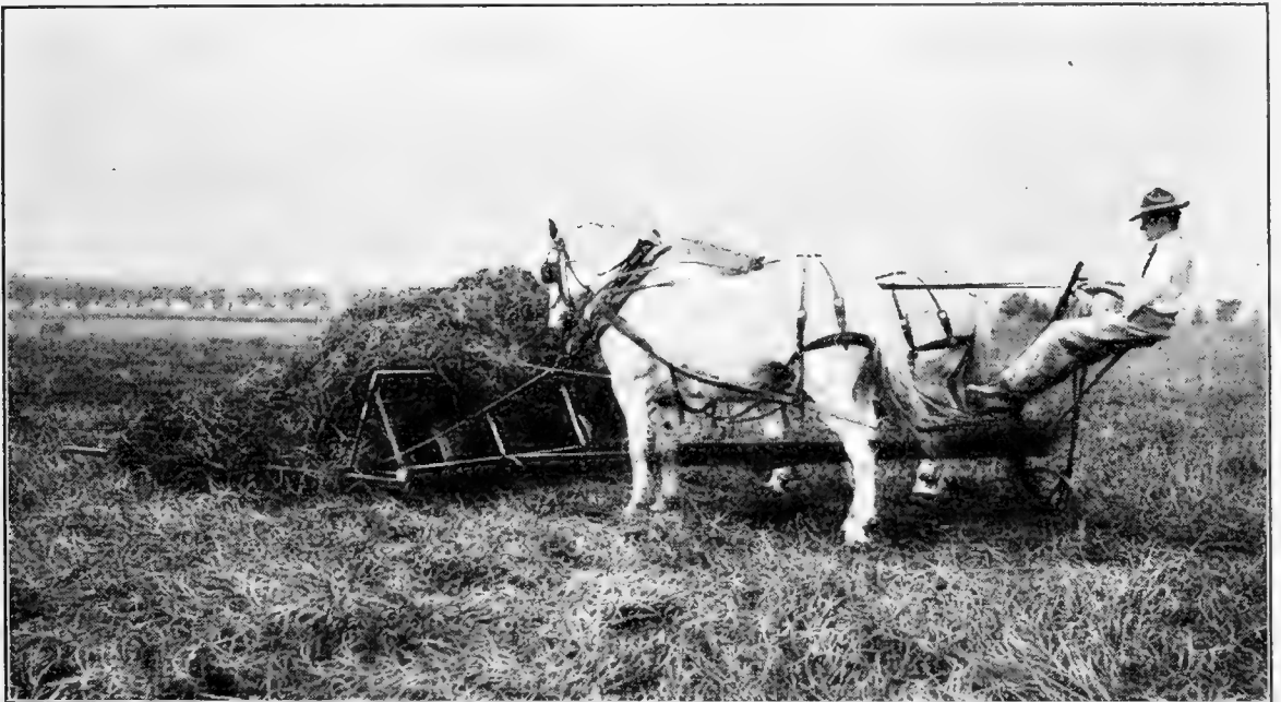
INTERNATIONAL REAR HITCH SWEEP RAKE IN THE FIELD.
