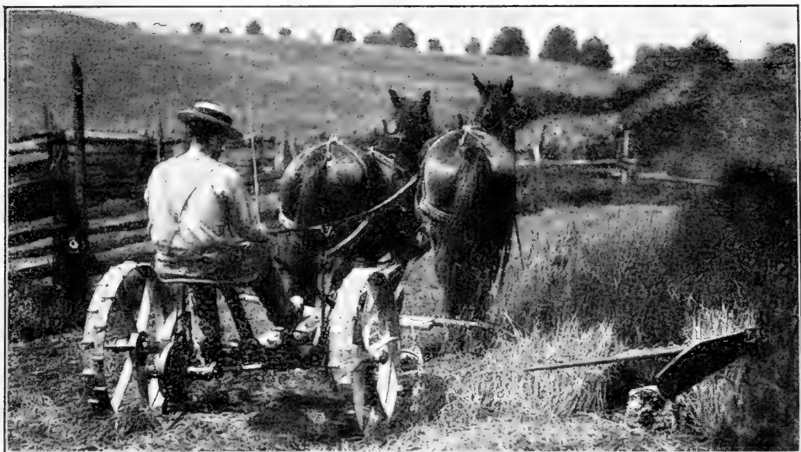
DEERING MOWER PASSING AN OBSTRUCTION.
