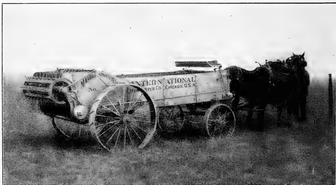
INTERNATIONAL HARVESTER COMPANY ENDLESS APRON MANURE SPREADER "CLOVERLEAF" BEFORE LOADING FOR THE FIELD.
