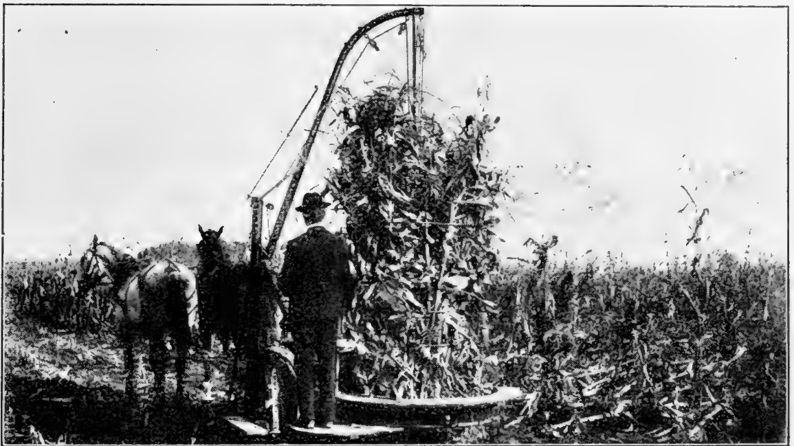
CORN SHOCKER CUTTING AND GATHERING THE SHOCK.
