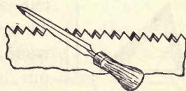
FIG. 165.—POSITION OF FILE IN FILING A SAW.
