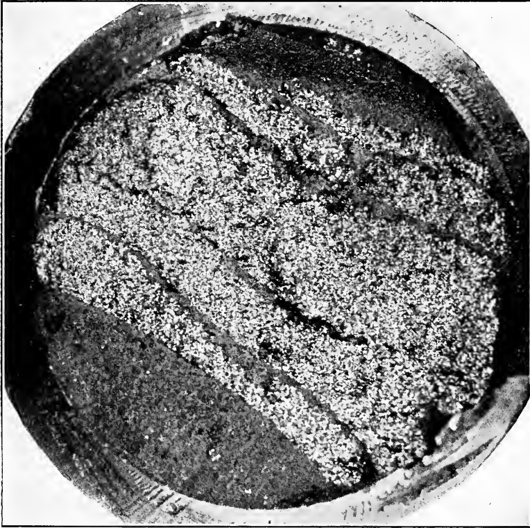
FIG. 86.—Fatigue fracture of bolt under repeated axial tension.
