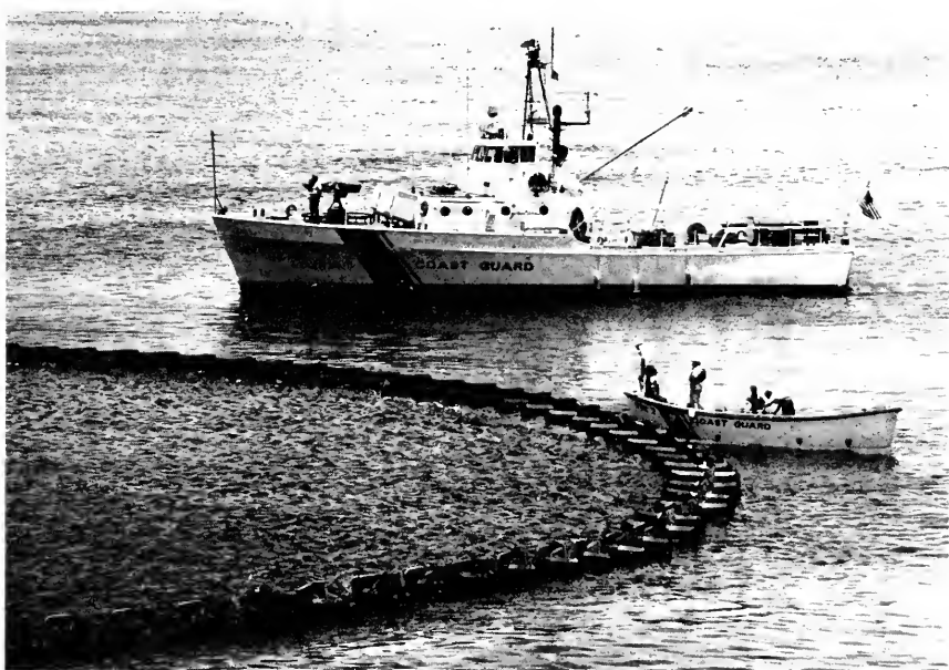
As the Coast Guard Cutter Point Thatcher stands by, marine engineers test an experimental floating oil barrier during a simulated oil spill. Soybean oil, which is nontoxic and biodegradable, is used in place of crude oil.
