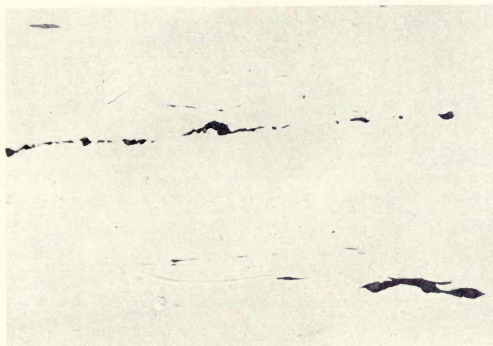
FIG. 61—Silicate or slag inclusions (with a few gray sulphides) in the cross section of the web of a rail.
