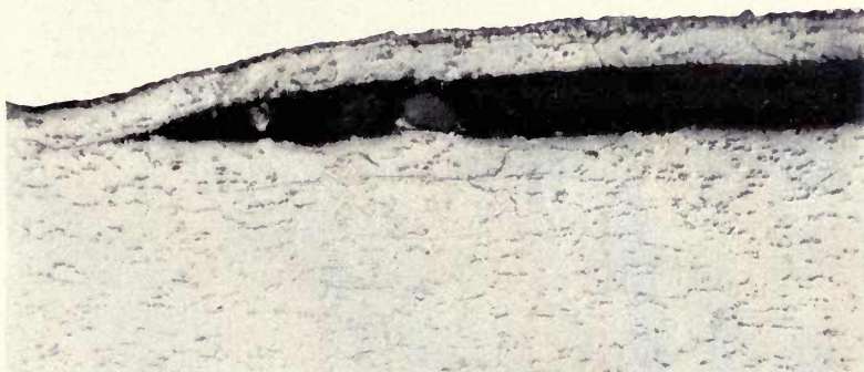
FIG. 40 — Section through one of the blisters shown in Fig. 38, magnified 200 diameters, showing traces of oxide remaining in the blister.
