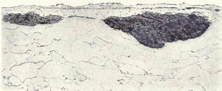
FIG. 36 — Section of sheet shown in Fig. 35, magnified 200 diameters, showing large slag enclosures just below the steel surface.
