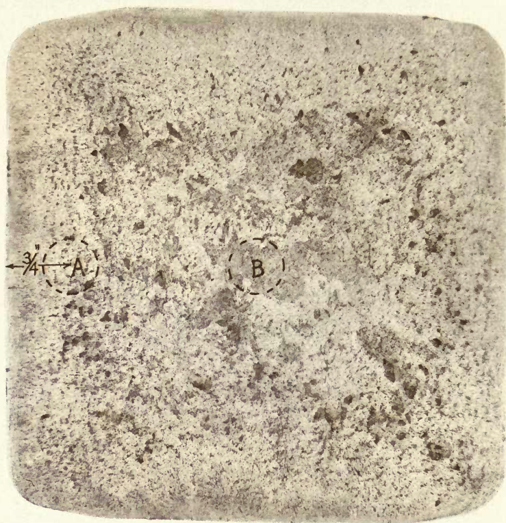
FIG. 14 — Sulphur print of heat No. 1, killed with aluminum.
