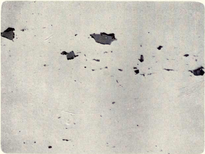
FIG. 56 — Longitudinal section of a low-carbon and low-manganese steel wire rod, magnified 200 diameters and unetched, showing a bad streak of slag (silicate) inclusions. Numerous cracks had started along other streaks like this in this sample.
