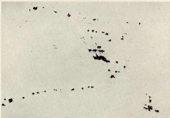
FIG. 66—Group of segregated inclusions in cross section of the web of a rail in which 0.003% of alumina was found by chemical analysis. Magnified 200 diameters.
