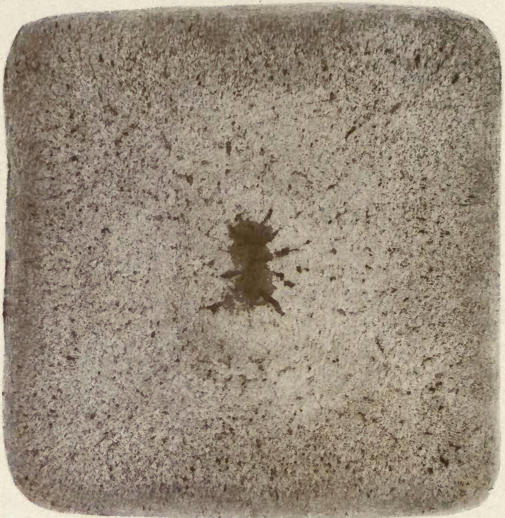
FIG. 11 — Sulphur print of segregated untreated forging steel.
