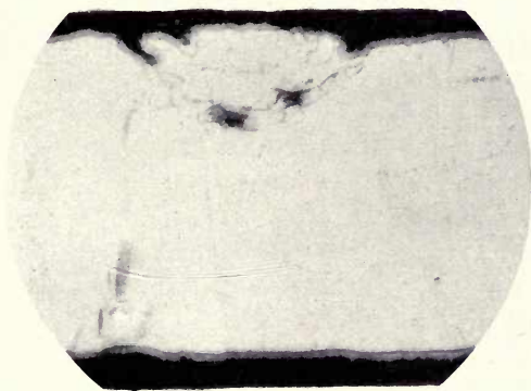
FIG. 34 — Section of galvanized sheet with "gray coating," showing uneven steel surface that caused the small spangle. The zinc has been blackened in this case by ammonia.
