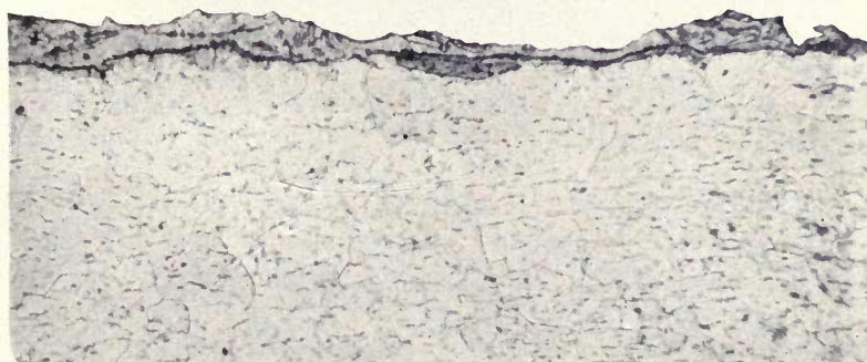
FIG. 32 — Section of sheet shown in Fig. 29, magnified 200 diameters, showing impurity in the tin, causing an uneven coating.
