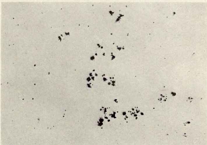
FIG. 62—Alumina inclusions in a soft steel ingot in which more alumina was found by chemical analysis than all other oxides.
