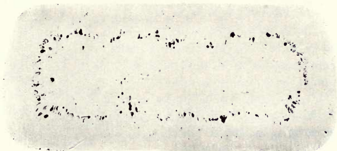
FIG. 44 — Polished section of ingot 14x30 inches.
