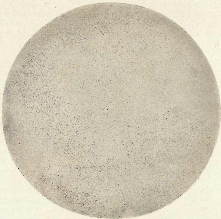
FIG. 13 — Sulphur print of titanium treated 8-inch axle, showing entire absence of segregation.
