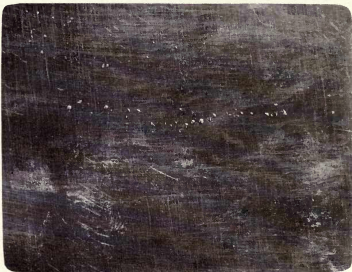
FIG. 38 — Natural size photograph of a typical blistered tin sheet.
