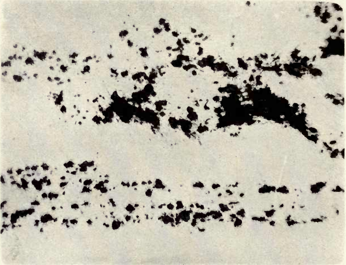
FIG. 16 — Photomicrograph of a longitudinal section of a billet of heat No. 1 (Fig. 14), cut midway between center and edge, unetched, and magnified 200 diameters, showing part of a long streak of alumina particles.
