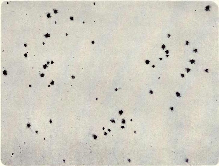
FIG. 55 — Cross-section of a high-carbon steel wire rod, magnified 200 diameters and unetched, the inclusions of alumina showing clearly that aluminum was used in treating this steel.
