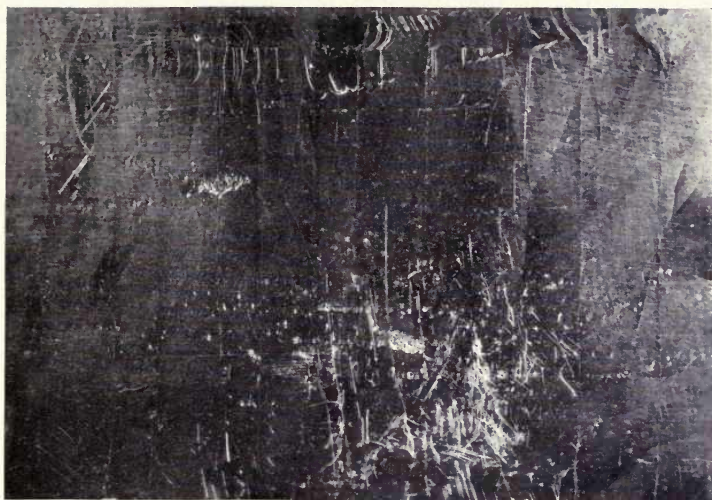
FIG. 35 — Natural size photograph of surface of a tinned sheet in which slag was found below the defective spots.
