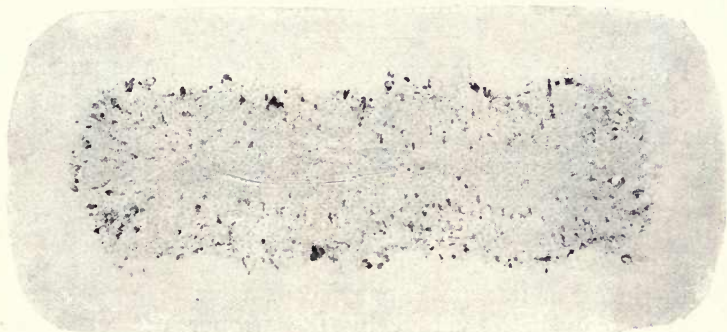
FIG. 45 — Sulphur print of ingot 14x30 inches.
