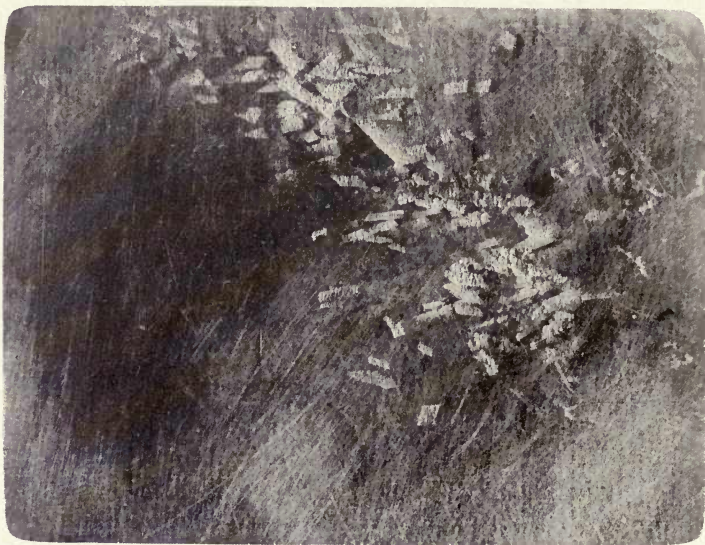
FIG. 28 — Natural size photograph of tinned sheet showing defective surface.
