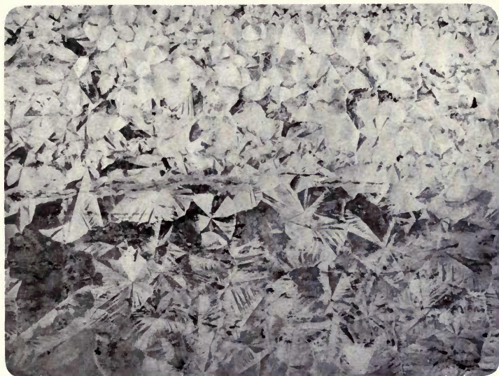
FIG. 33 — Natural size photograph of a "gray coating," showing variation in size of spangle on a galvanized sheet.
