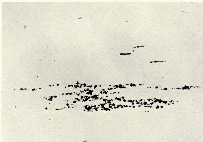
FIG. 60—Inclusions of alumina in section parallel to direction of forging of steel treated with a large excess of aluminum. The few gray spots are sulphides.
