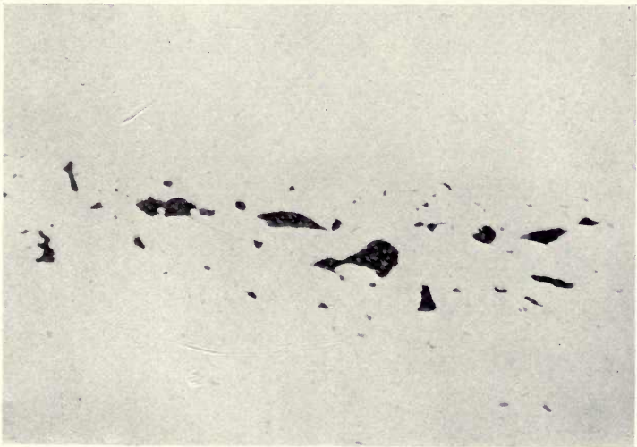
FIG. 73—Slag inclusions in similar steel treated with oxide of titanium before casting. BOTH SHOW LONGITUDINAL SECTIONS OF THE FORGED ENDS OF SMALL INGOTS CAST FROM 10-LB. MELTS OF THE SAME STEEL, UNETCHED AND MAGNIFIED 200 DIAMETERS
