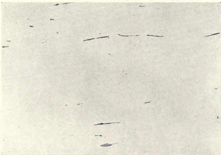
FIG. 10 — Typical small sulphide and silicate fibres in a billet of forging steel treated with titanium. Section cut parallel to direction of rolling, not etched, and magnified 200 diameters.
