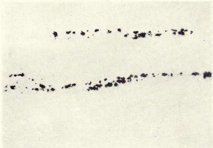
FIG. 9 — Streaks of alumina in a billet of forging steel deoxidized with aluminum. Section cut parallel to direction of rolling, not etched, and magnified 200 diameters.
