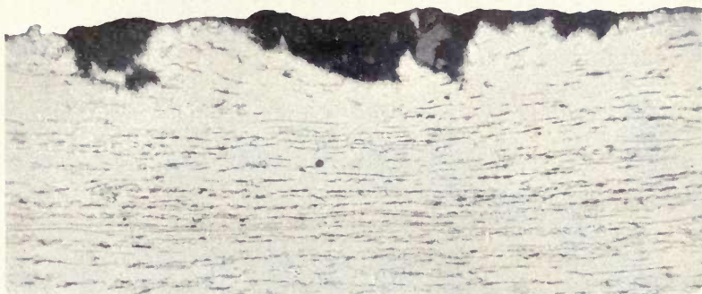
FIG. 30 — Section through one of the spots shown on Fig. 27, magnified 200 diameters, showing scale on the surface interrupting the tin coating.
