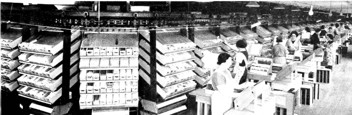
A section of the conveyor, 900 feet long, in one of the Detroit warehouses. During the busy seed packing season, nearly one million packets are picked out daily in filling FERRY'S Red-and-Silver Displays
