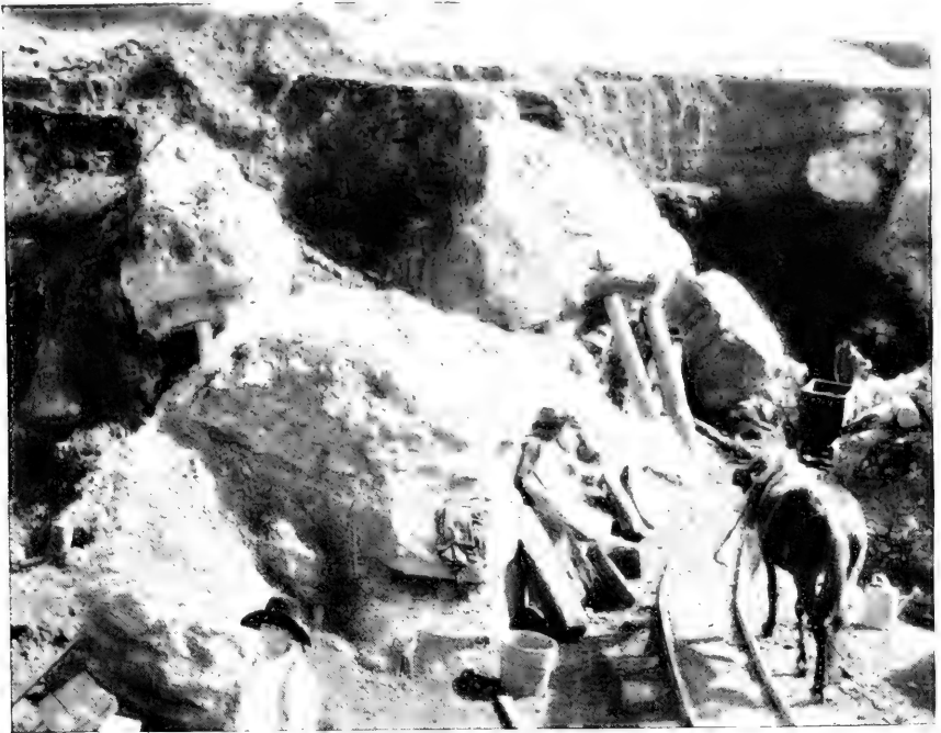
FIG. 2.—BROWN-ROCK MINING, SHOWING BOWLERS OF PHOSPHATIC LIMESTONE.
