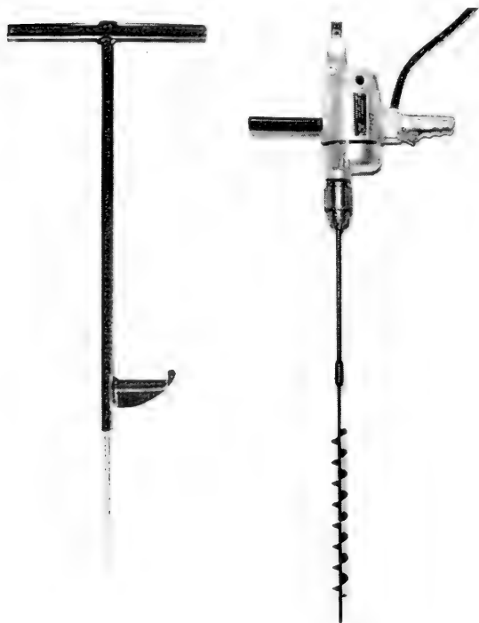
Fig. 6.—A punch bar (left) or an electric drill with a soil auger (right) can be used to prepare holes for application of dry phosphorus and potassium fertilizers.
