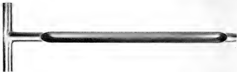
Fig. 3.—The soil profile tube is a handy tool for removing cores of soil from the upper 10–14 inches. Many properties of the soil can be observed by examining such cores.
