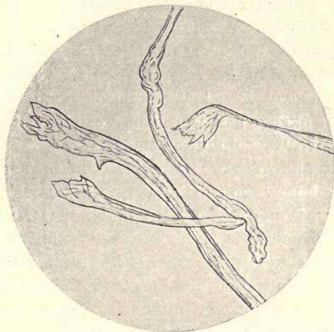
FIG. 39.—Cotton after Treatment with Sodium Hypochlorite Solution.
