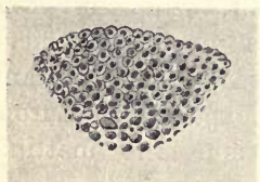
FIG. 60.—Portion of Cross-section through Coconut Fibre.
