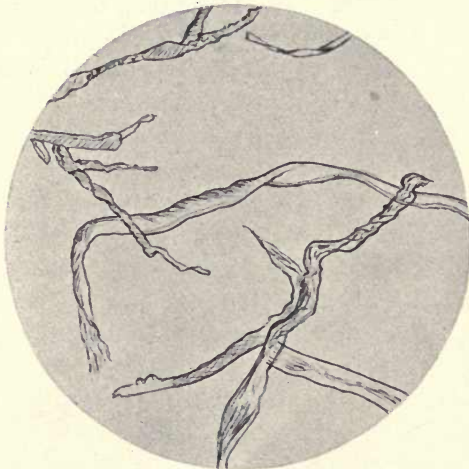
FIG. 40.—Cotton Fibres Disintegrated by Mould.
