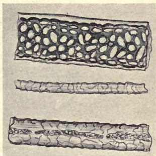
FIG. 1.—Structure of Wool Fibre. Scotch Black-faced Sheep.
