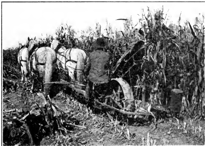
Fig. 30. The corn binder for cutting corn for fodder or silage. Much corn is also cut by hand or by some form of cutter which does not bind it into bundles.
