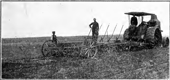
Fig. 49. Plowing, seeding, and harrowing at one operation. A common method of sowing wheat on the large wheat farms of the Western states.
