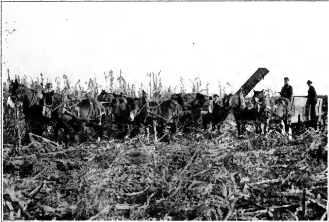
Fig. 27. The corn picker, a machine for gathering the ears from standing corn. Not yet in general use.
