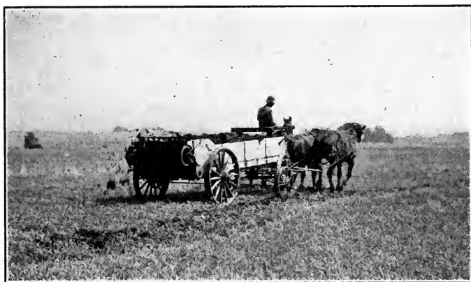
Fig. 153. The manure spreader distributes the manure evenly over the soil so that it can be plowed under without trouble and placed where it will be most easily reached by crops. The easiest way to handle manure is to load it directly into the spreader from the stable.
