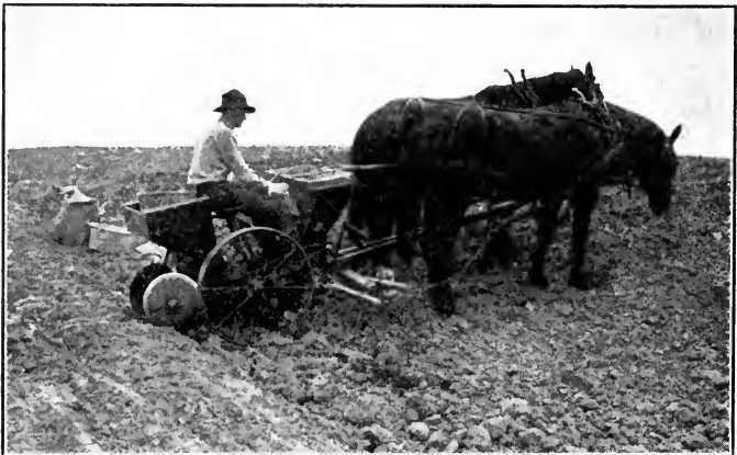
Fig. 134. The potato planter. A good machine to use where several acres of this crop are to be planted.
