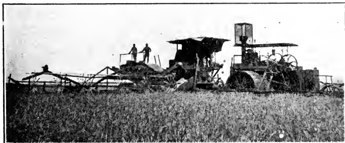
Fig. 55. Combined harvester and thrasher drawn by traction engine. A machine of the same type as that shown in Fig. 51.
