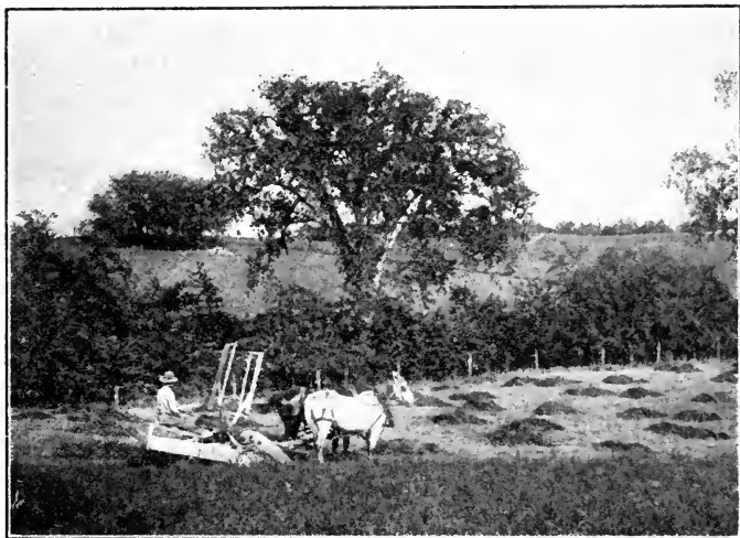
Fig. 120. Cutting alfalfa for seed with the self-rake reaper. This machine is still used in some sections for harvesting grain. It deposits the crop in bunches, as shown at the right in the picture.
