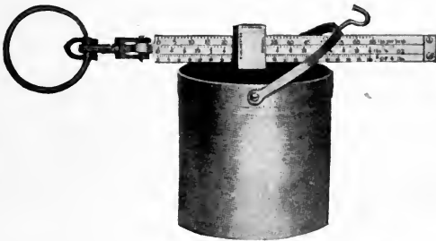
FIG. 27.—Kettle for Determining the Weight per Measured Bushel. The Vessel Should be Filled to Overflowing by Pouring the Grain from a Bag Held about Two Inches above the Top. Before Weighing the Grain is Leveled Off by a Diagonal Stroke.
