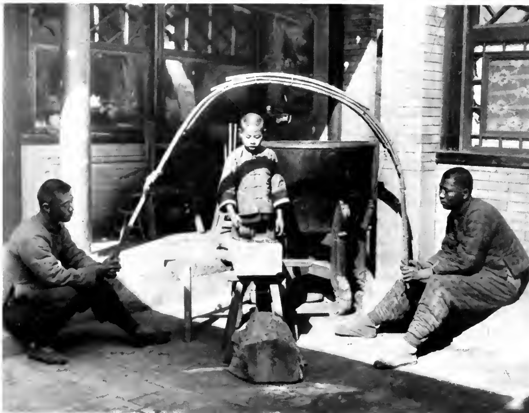
Photo taken in China in the early years of this century shows two jade cutters at the time-consuming process of slicing through a large block of this hard material.
