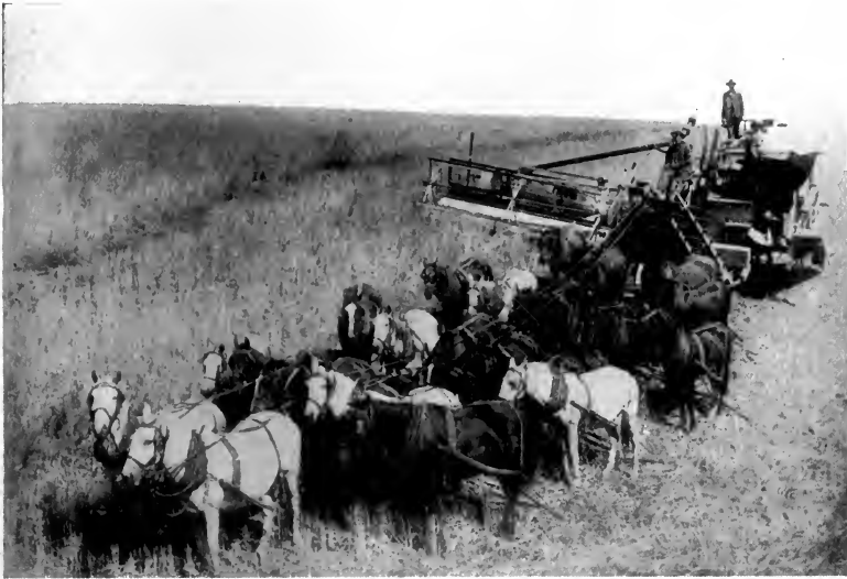
Cutting, binding, and threshing all at once
