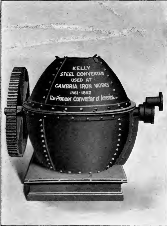
The First Pneumatic Converter Used in the United States. Photographed on the Lawn of the Cambria Steel Company Offices in Johnstown, Pa., Where It is Preserved as a Curiosity.
