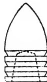
390 GRAIN HOLLOW BASE BULLET FOR .54 CAL. RIFLES, HARPERS FERRY, 1849-1855 FOR USE IN MODELS 1841, '42
