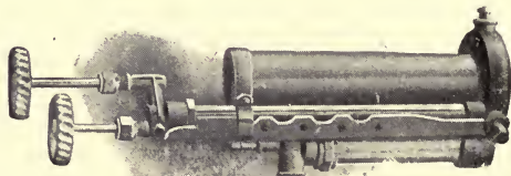
FIG. 18. GASOLINE ASSAY FURNACE WITH TANK AND BURNER.
